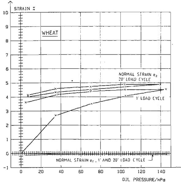
Fig. 9. Strain state in wheat filled calibration chamber
