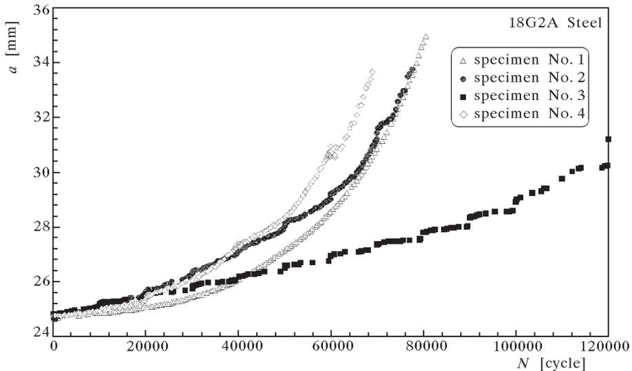
Fig. 2. Crack length  $a$  vs. number of cycles  $N$  for CT specimens made of 18G2A steel under fatigue tests with overloads applied in cycles
