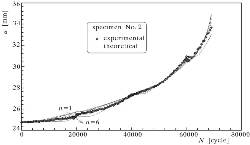
Fig. 3. Theoretical description of crack propagation in CT specimens made of 18G2A steel
