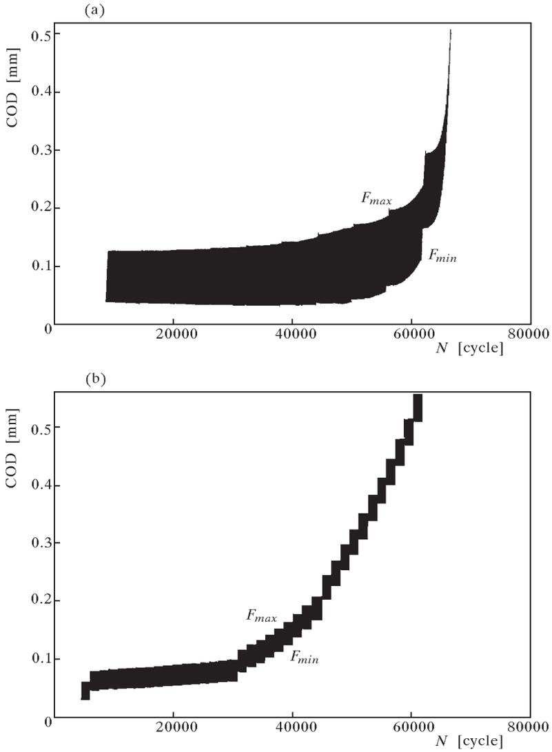
Fig. 1. Experimental records of crack opening displacement in CT specimen made of PA7 duralumin under fatigue tests with overloads applied in cycles
