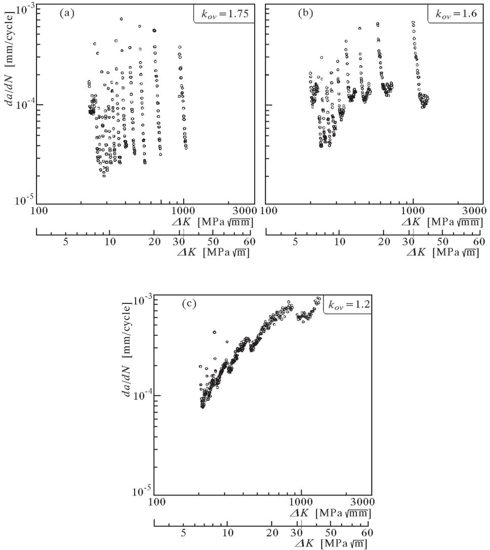
Fig. 5.  $da/dN = f(\Delta K)$  relationship for specimen tested with overload  $k_{ov} = 1.75, 1.6, 1.2$
