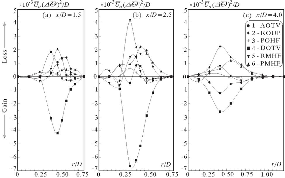
Fig. 1. Budget of oscillatory component of temperature variance at the cross-sections: (a)  $x/D = 1.5$ , (b)  $x/D = 2.5$ , (c)  $x/D = 4.0$
