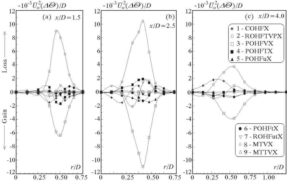
Fig. 10. Budget of oscillatory heat fluxes of longitudinal component, at the cross-sections: (a)  $x/D = 1.5$ , (b)  $x/D = 2.5$ , (c)  $x/D = 4.0$
