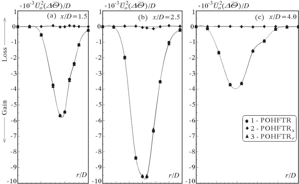
Fig. 15. Radial distributions of axial, radial and total production of radial, oscillatory heat fluxes performed by mean temperature component at the cross-sections: (a)  $x/D = 1.5$ , (b)  $x/D = 2.5$ , (c)  $x/D = 4.0$
