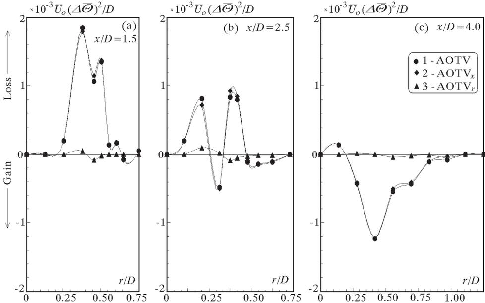
Fig. 2. Radial distributions of axial, radial and total advection of oscillatory component of temperature variance at the cross-sections: (a)  $x/D = 1.5$ , (b)  $x/D = 2.5$ , (c)  $x/D = 4.0$
