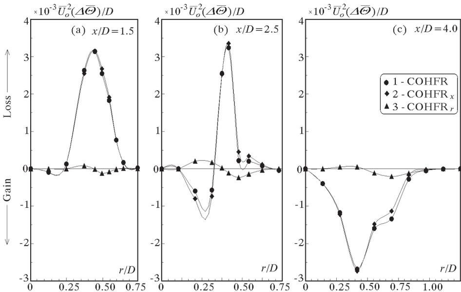
Fig. 13. Radial distributions of axial, radial and total advection of radial oscillatory heat fluxes at the cross- sections: (a)  $x/D = 1.5$ , (b)  $x/D = 2.5$ , (c)  $x/D = 4.0$
