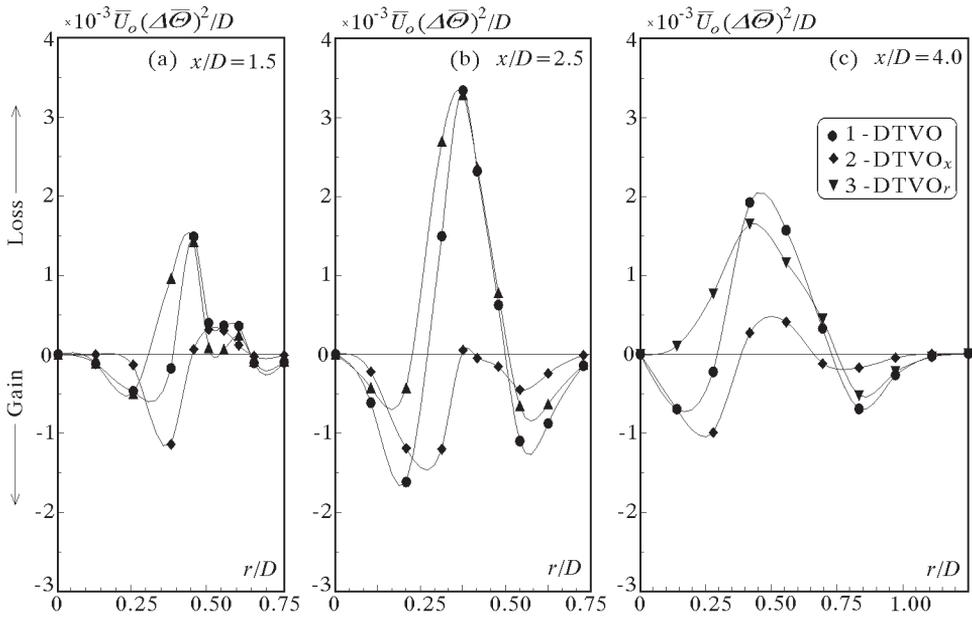
Fig. 8. Radial distributions of axial, radial and total diffusion of random component of temperature variance performed by oscillatory motion at the cross-sections: (a)  $x/D = 1.5$ , (b)  $x/D = 2.5$ , (c)  $x/D = 4.0$
