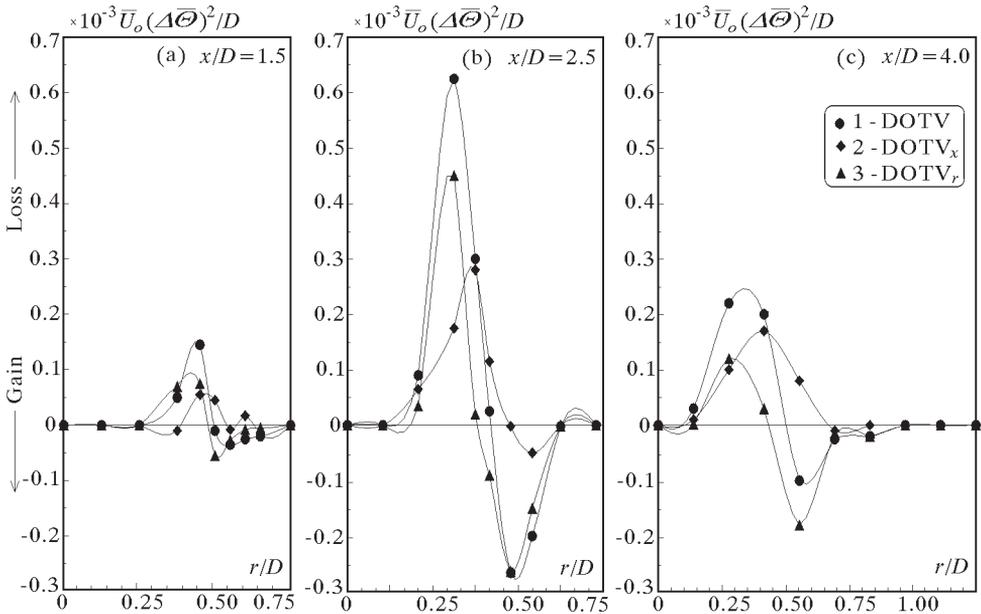
Fig. 3. Radial distributions of axial, radial and total diffusion of oscillatory component of temperature variance at the cross-sections: (a)  $x/D = 1.5$ , (b)  $x/D = 2.5$ , (c)  $x/D = 4.0$
