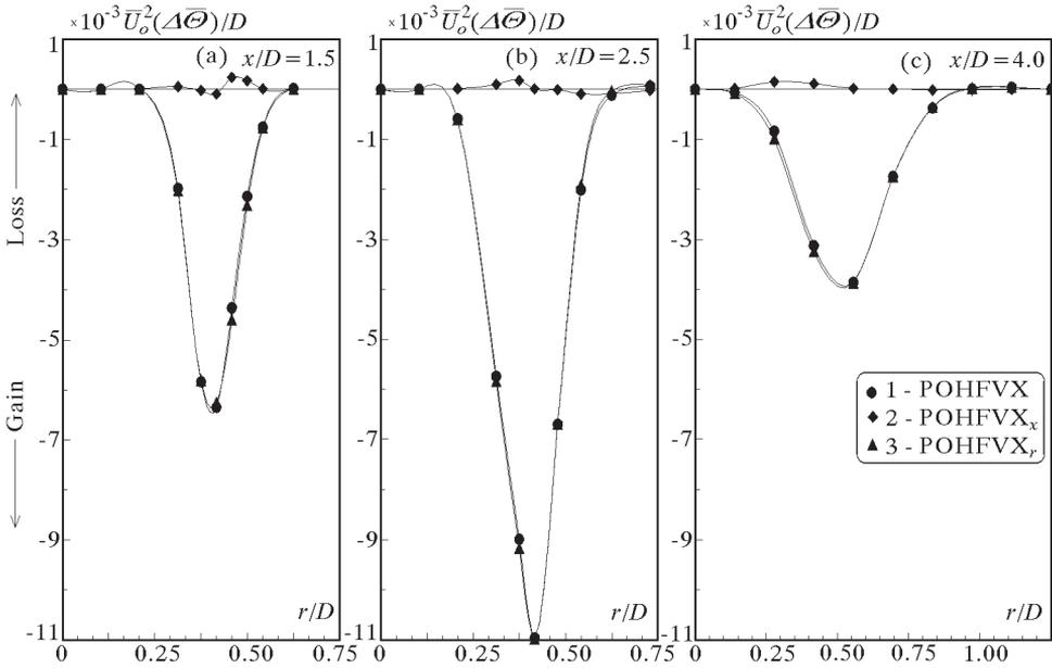
Fig. 14. Radial distributions of axial, radial and total production of axial, oscillatory heat fluxes realised by longitudinal component of mean velocity component, at the cross-sections: (a)  $x/D = 1.5$ , (b)  $x/D = 2.5$ , (c)  $x/D = 4.0$
