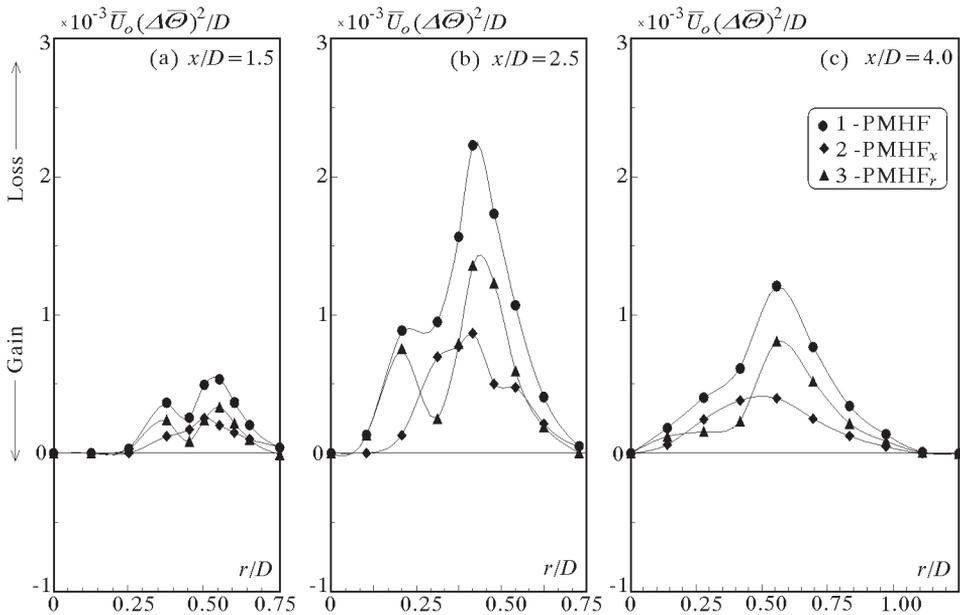
Fig. 5. Radial distributions of axial radial and total production of oscillatory component of temperature variance performed by modulated heat fluxes, at the cross-sections: (a)  $x/D = 1.5$ , (b)  $x/D = 2.5$ , (c)  $x/D = 4.0$
