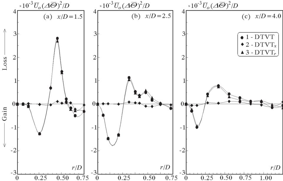
Fig. 7. Radial distributions of axial, radial and total diffusion of random component of temperature variance performed by turbulent motion at the cross-sections: (a)  $x/D = 1.5$ , (b)  $x/D = 2.5$ , (c)  $x/D = 4.0$
