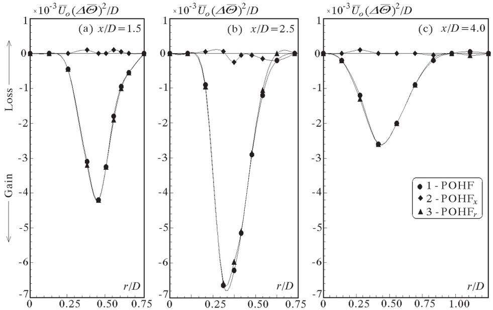
Fig. 4. Radial distributions of axial radial and total production of oscillatory component of temperature variance performed by oscillatory heat fluxes, at the cross-sections: (a)  $x/D = 1.5$ , (b)  $x/D = 2.5$ , (c)  $x/D = 4.0$
