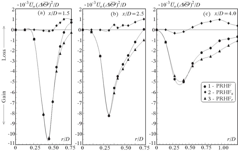
Fig. 9. Radial distributions of axial radial and total production of random component of temperature variance performed by turbulent heat fluxes, at the cross-sections: (a)  $x/D = 1.5$ , (b)  $x/D = 2.5$ , (c)  $x/D = 4.0$
