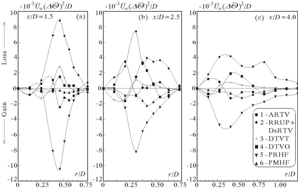
Fig. 6. Budget of random component of temperature variance at the cross-sections: (a)  $x/D = 1.5$ , (b)  $x/D = 2.5$ , (c)  $x/D = 0.4$
