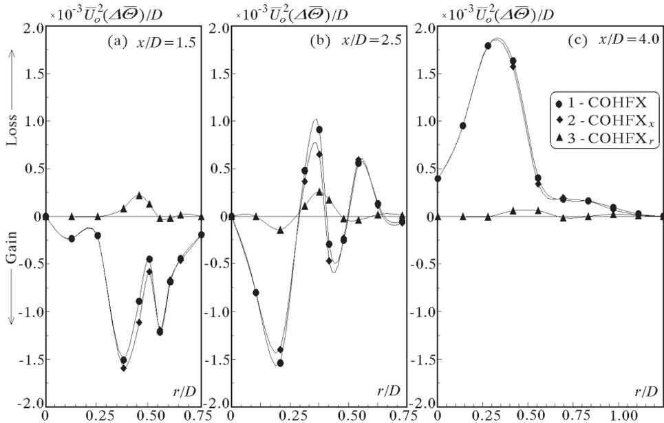
Fig. 12. Radial distributions of axial, radial and total advection of axial oscillatory heat fluxes at the cross- sections: (a)  $x/D = 1.5$ , (b)  $x/D = 2.5$ , (c)  $x/D = 4.0$
