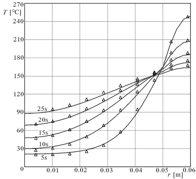
Fig. 7. Temperature field in domain considered ( $\Delta t = 1.25$  s)
