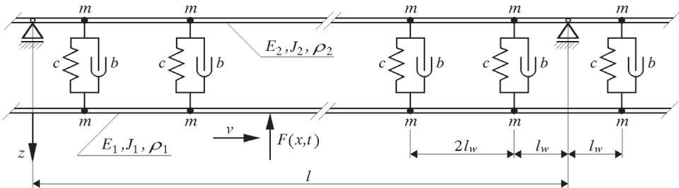
Fig. 2. The catenary model: two visco-elastically connected Bernoulli-Euler beams with concentrated masses. The upper beam rigidly supported on the foundation
