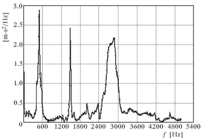
Fig. 8. Spectral density of the free horizontal vibration acceleration of the pantograph model beam (impact horizontal excitation, piezoelectric accelerometer)
