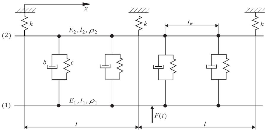
Fig. 1. The catenary model: two visco-elastically connected Bernoulli-Euler beams with the upper finite elastically supported
