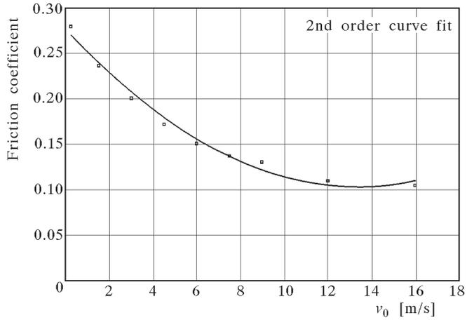
Fig. 9. Exemplary results of investigations on dynamic friction coefficient (in function to relative slip velocity)
