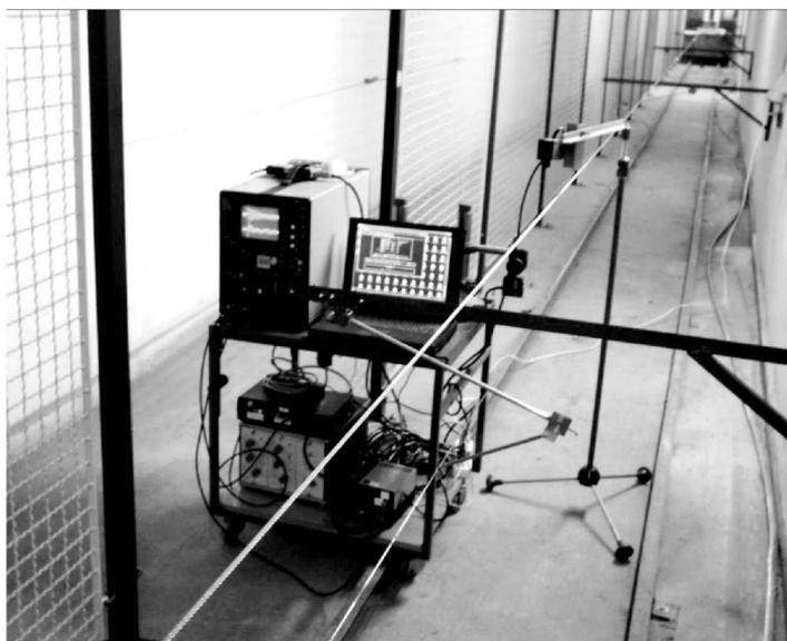
Fig. 6. Facility for testing natural frequencies and modes of vibrations of the catenary system of a physical model
