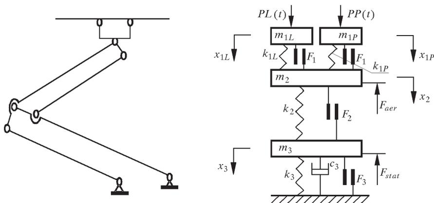
Fig. 3. Reduced physical model of a real pantograph system
