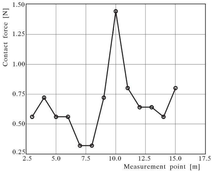
Fig. 10. Exemplary results of the contact force measurements (mean distribution along the wire)
