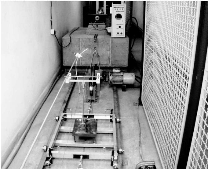
Fig. 7. A rail-car with the model of pantograph; in the background the elements of the driving system: guiding wheels, cable rewinding, electric engine can be seen
