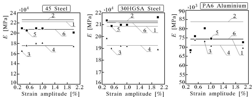
Fig. 7. Values of the modulus  $E$ ; 1 –  $E$  (static) linear approximation, 2 –  $E$  (static) tangent, 3 –  $E_d$  (dynamic) linear, 4 –  $E_d$  linear-mean, 5 –  $E_d$  (dynamic) tangent, 6 –  $E_d$  tangent-mean
