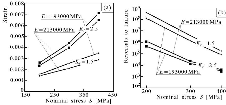
Fig. 11. Changes of the local strain (a), fatigue life for strain-based calculations (b) for 30HGSA Steel
