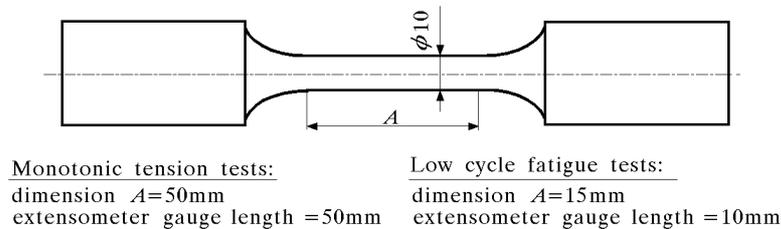
Fig. 5. Specimens used in the investigations
