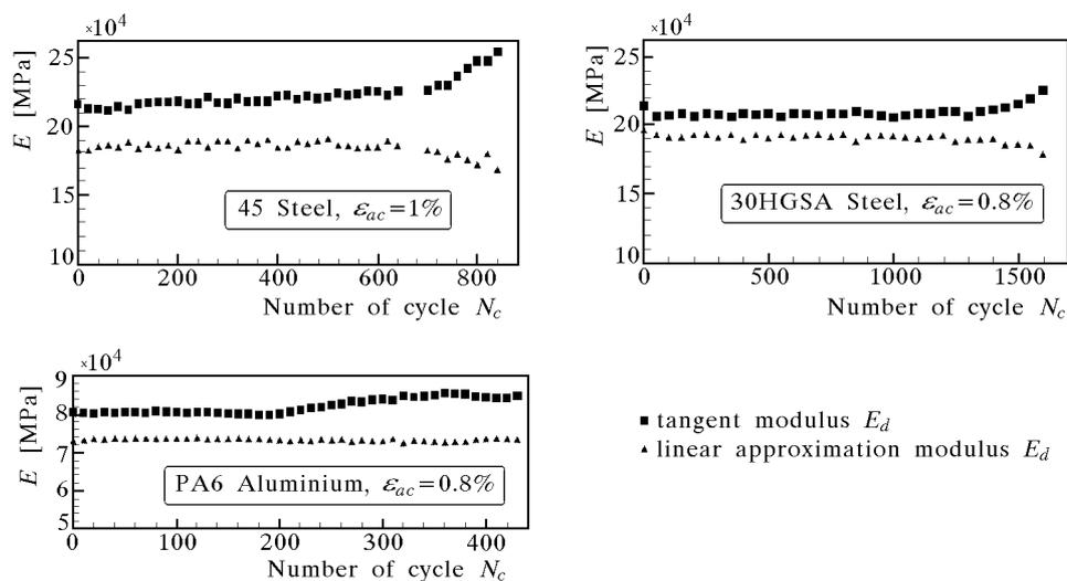
Fig. 8. Exemplary courses of the modulus  $E$  for specimens made of the three tested materials
