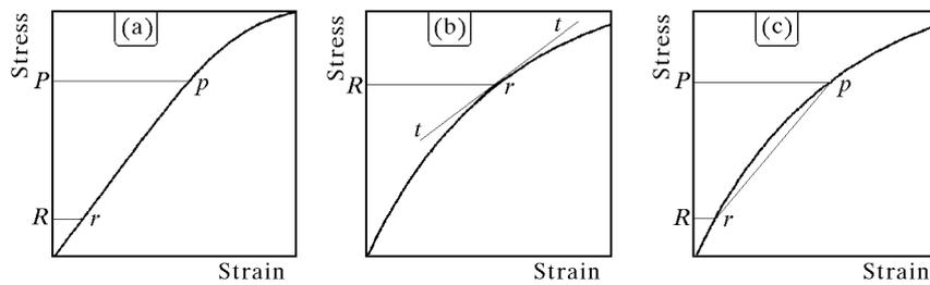
Fig. 4. Methods of determination of the elasticity modulus: (a) linear, (b) tangent, (c) secant
