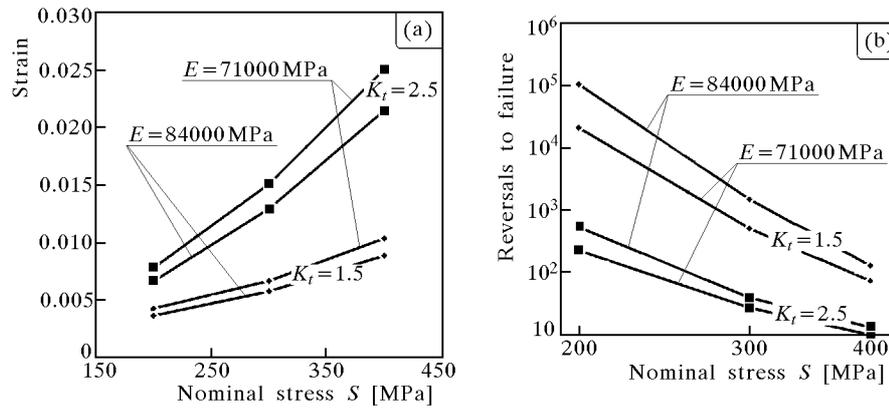
Fig. 12. Changes of the local strain (a), fatigue life for strain-based calculations (b) for PA6 Aluminium
