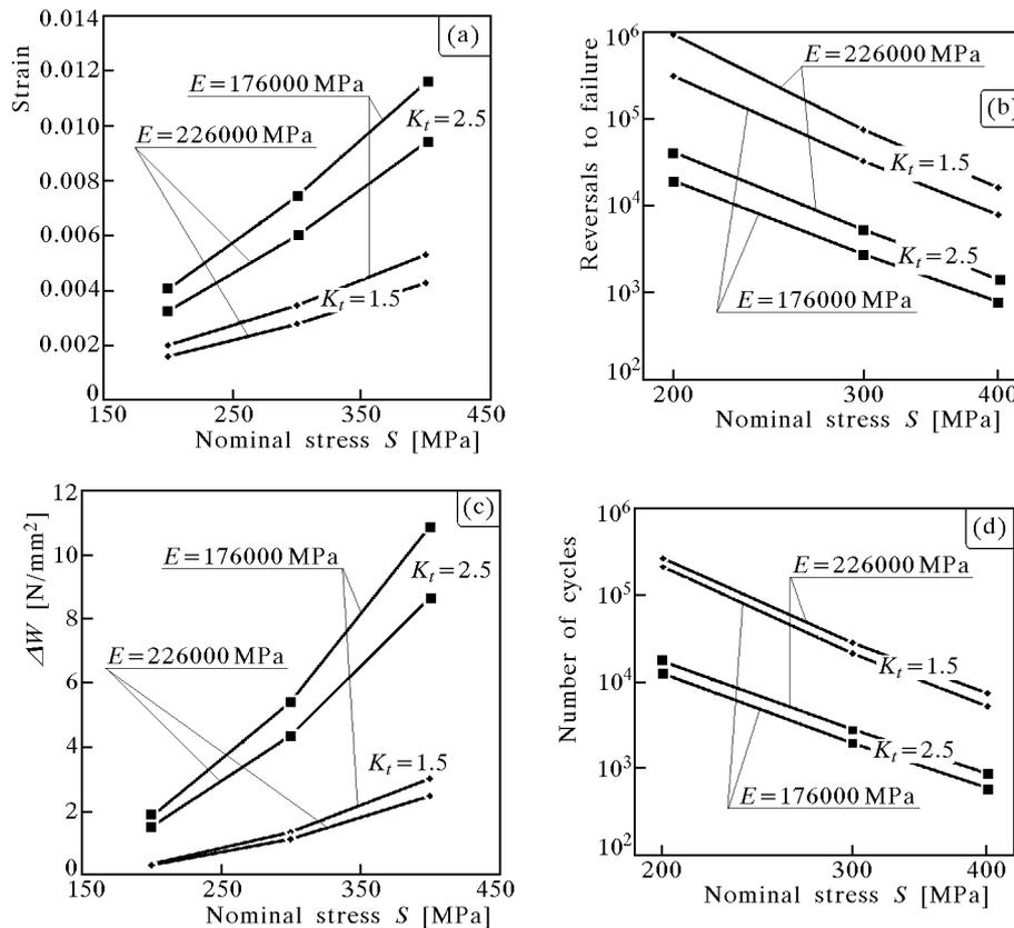
Fig. 10. Changes of the local strain (a), plastic strain energy (c), fatigue life for strain-based calculations (b) and energy based calculations (d) for 45 Steel
