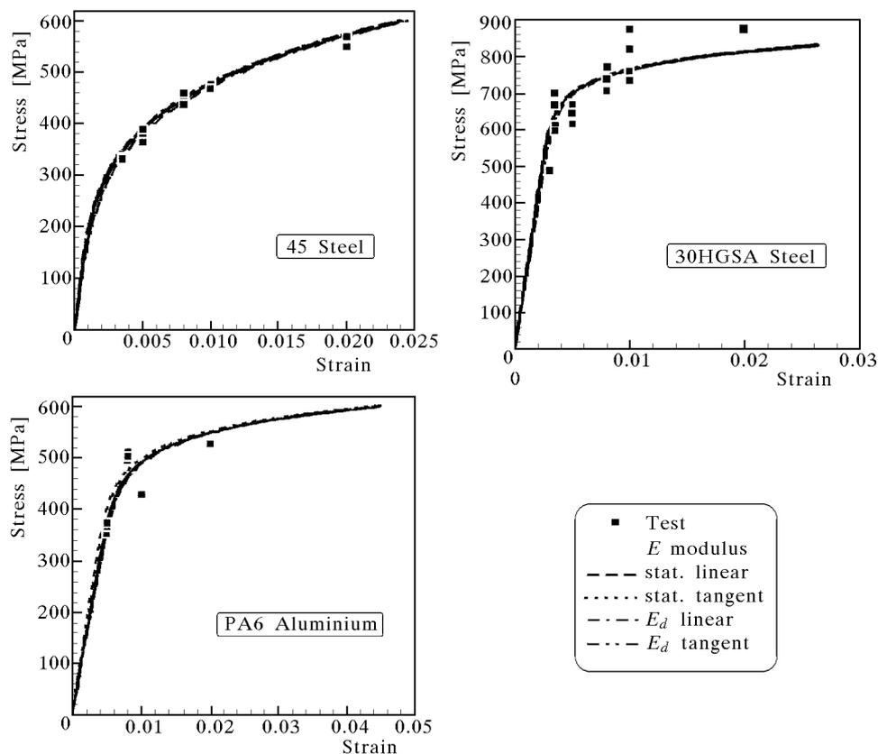
Fig. 9. Stress-strain curves for different values of the modulus  $E$
