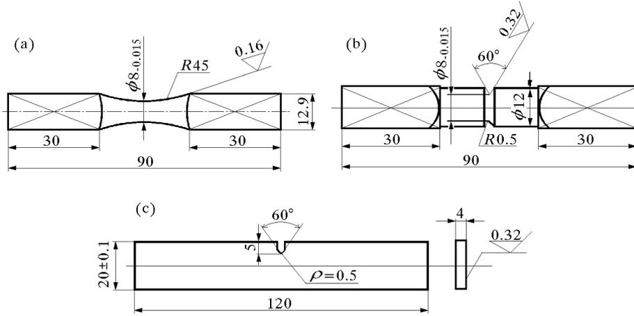
Fig. 1. Specimens subjected to tests, (a) round, (b) round notched, (c) flat notched
