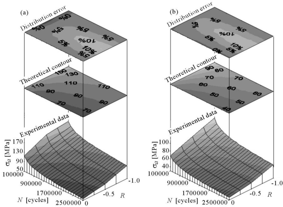
Fig. 3. The limiting stress surface under bending determined from tests, the theoretical contour and error distribution, (a) flat notched specimens – 18G2A, (b) flat notched specimens – PA6
