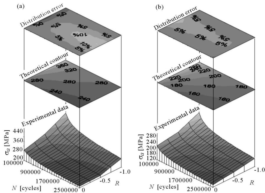
Fig. 2. The limiting stress surface under bending determined from tests, the theoretical contour and error distribution, (a) round specimens – 18G2A, (b) round notched specimens – 18G2A
