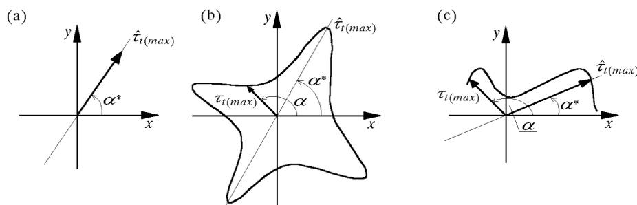
Fig. 2. The distinguished states of the maximum shear stress vector; (a)  $\varphi = 0$ ,  $\sigma_{x(m)} = \tau_{xy(m)} = 0$ , (b)  $\varphi \neq 0$ ,  $\sigma_{x(m)} = \tau_{xy(m)} = 0$ , (c)  $\sigma_{x(m)} \neq 0$ ,  $\tau_{xy(m)} \neq 0$
