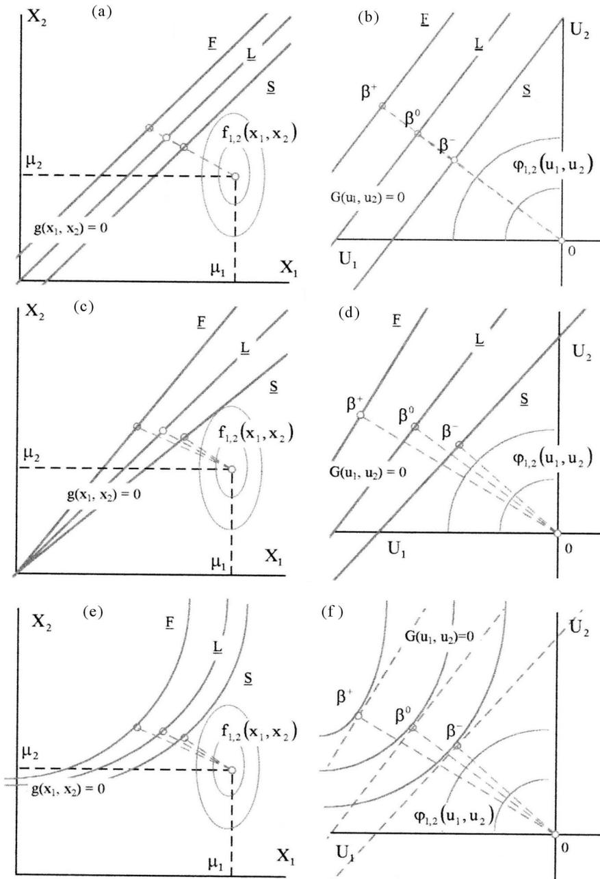
Fig. 5. Fuzzy areas of the failure  $\underline{F}$ , limit state  $\underline{L}$  and survival  $\underline{S}$  in the variables  $X_1, X_2$  and standard variables  $U_1, U_2$  coordinate systems
