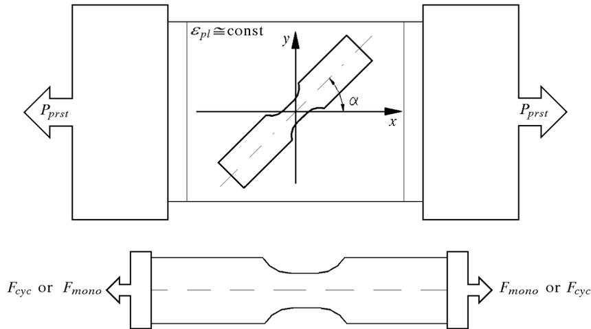
Fig. 1. The method of obtaining specimens for tests (Cichański and Sempruch, 2005)
