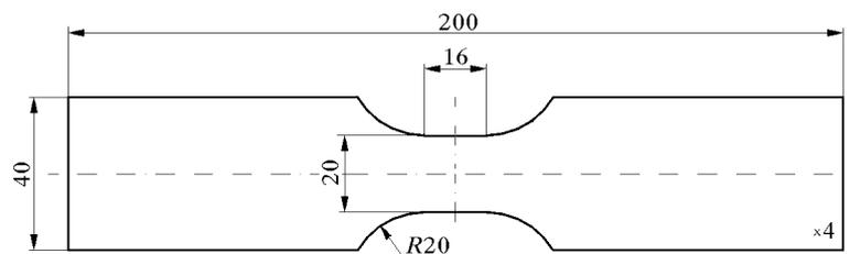
Fig. 3. Geometric shape of the specimen for the preliminary fatigue research
