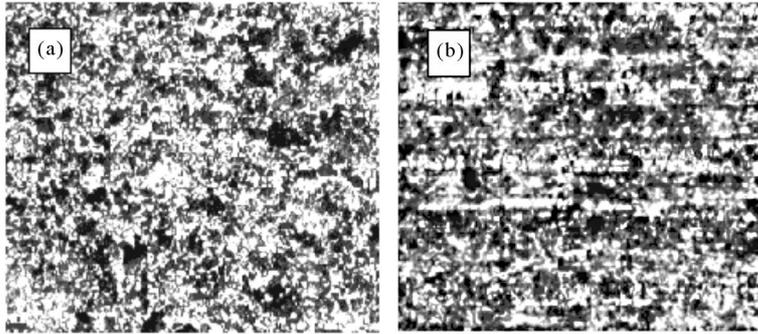
Fig. 6. Sheet metallographic structures: (a) near the surface; (b) in the middle of the intersection (multiplied by  $80\times$ )
