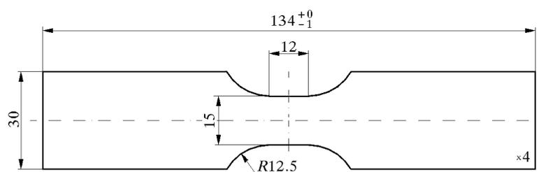
Fig. 4. Geometric shape of the specimen used in the main fatigue research
