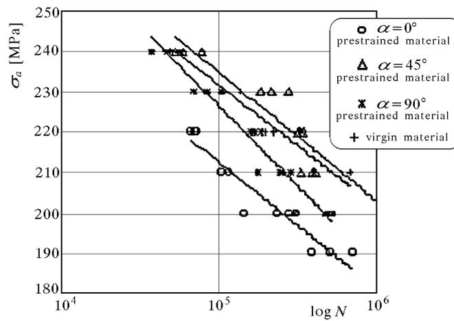
Fig. 12. Wöhler's line for the virgin and prestrained materials
