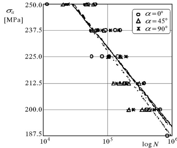
Fig. 8. Wöhler's lines for the virgin material
