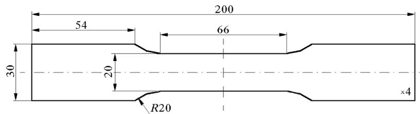
Fig. 2. Geometric shape of the specimen for determination of plastic properties
