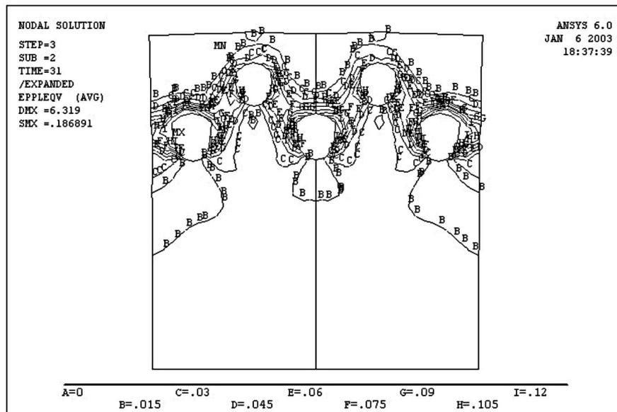
Fig. 5. The distribution of reduced plastic strains in the plate
