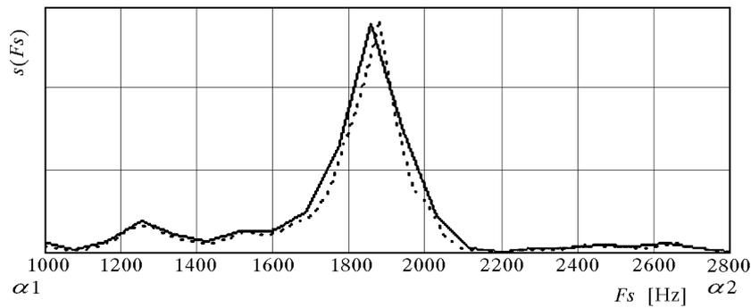
Fig. 5. Spectra of correctly – (full line) and wrongly cut off (broken line) signals – the main formant is shifted
