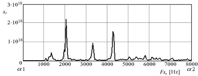
Fig. 1. Visualization of the signal spectrum in the frequency field of one of the investigated samples; the main formant occurs at a frequency of about 2050 Hz
