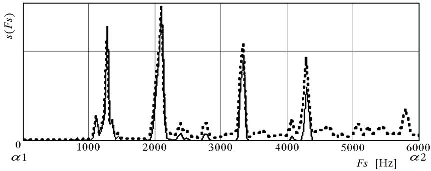
Fig. 2. An example of a signal spectrum with the use of a filter at the FFT stage (full line) as well as without the filter (broken line)
