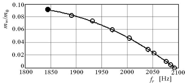
Fig. 8. A position characteristic of the main formants depending on the degree of material moisture – a cement plate
