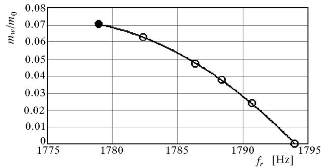
Fig. 7. A position characteristic of the main formants depending on the degree of material moisture – a sandstone plate
