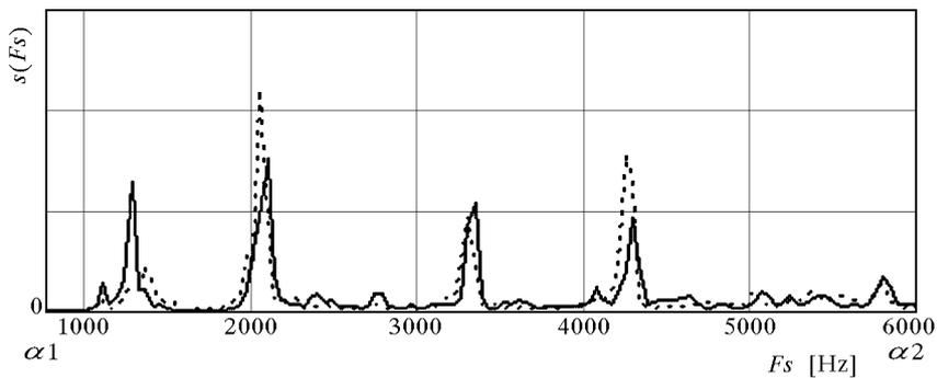
Fig. 6. A spectrum diagram of two signals of the object response to a percussive impulse – the object with different moisture
