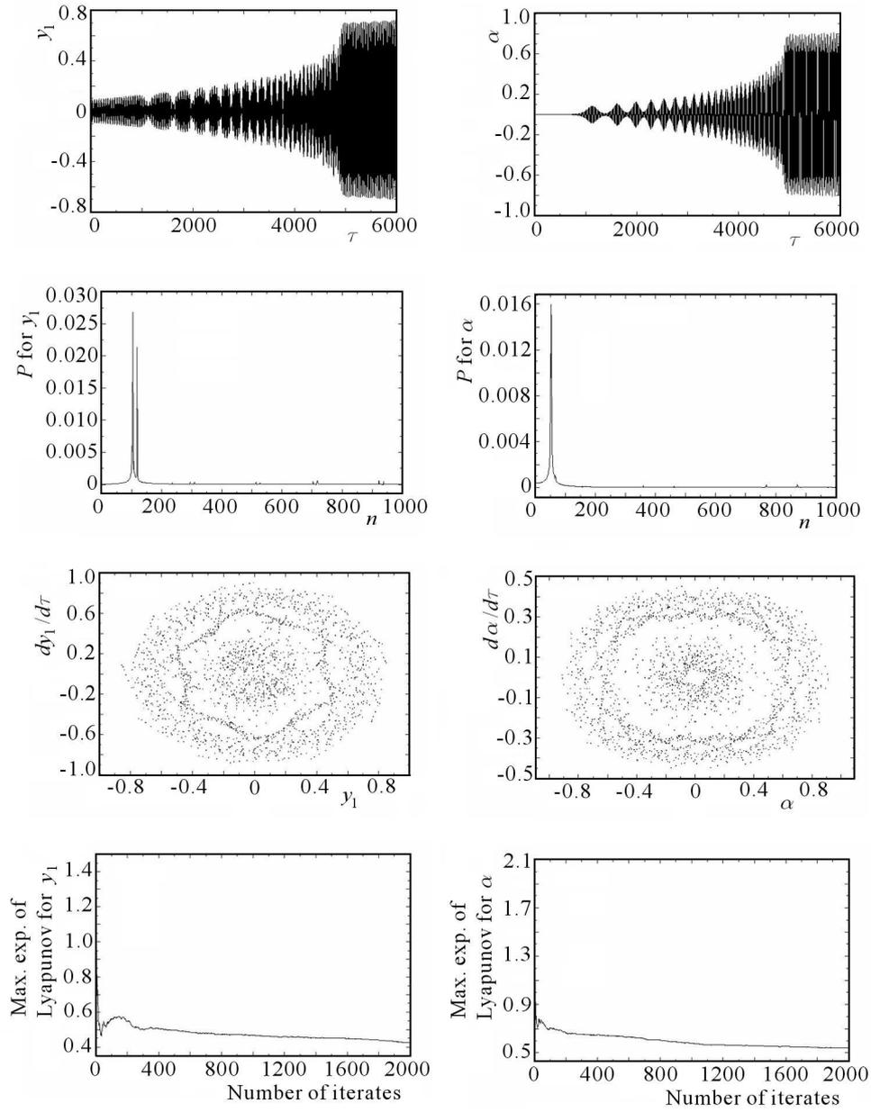
Fig. 7. Time histories, Power spectral densities, Poincaré's maps and maximum Lyapunov exponents corresponding to coordinate  $\alpha$  for the control parameter  $u_1 = 1.72$  and for:  $u_2 = 1.5$ ,  $q = 0.2$ ,  $\beta = 0.5$ ,  $a_1 = 0.01$ ,  $a_2 = 0.3$ ,  $\gamma_1 = 0.001$ ,  $\gamma_2 = \gamma_3 = \gamma_4 = 0$
