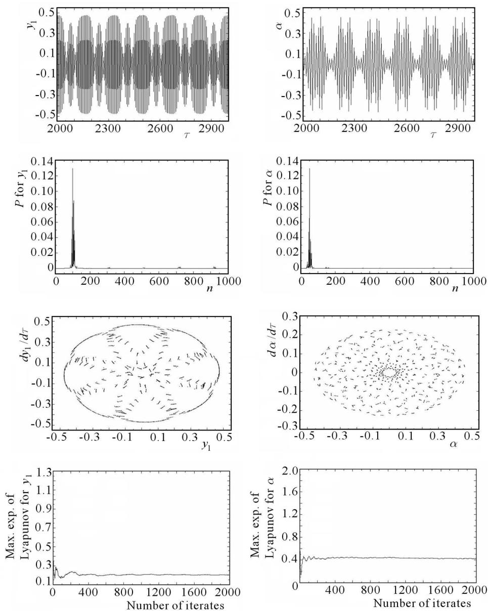
Fig. 6. Time histories, Power spectral densities, Poincaré's maps and maximum Lyapunov exponents corresponding to coordinates  $y_1$  and  $\alpha$  for the control parameter  $u_1 = 1.504$  and for:  $u_2 = 1.5$ ,  $q = 0.2$ ,  $\beta = 0.5$ ,  $a_1 = 0.01$ ,  $a_2 = 0.3$ ,  $\gamma_1 = 0.001$ ,  $\gamma_2 = \gamma_3 = \gamma_4 = 0$
