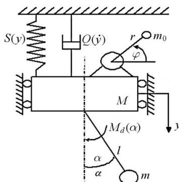
Fig. 1. A non-ideal model of an autoparametrical system
