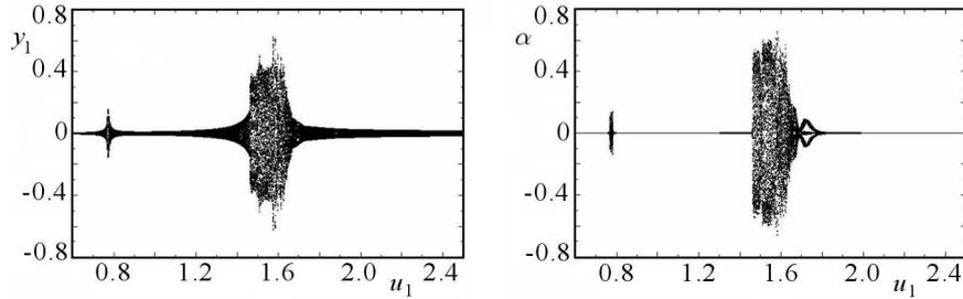
Fig. 3. Bifurcation diagrams for  $y_1$  and  $\alpha$  for:  $u_2 = 1.5$ ,  $q = 0.2$ ,  $\beta = 0.5$ ,  $a_1 = 0.01$ ,  $a_2 = 0.3$ ,  $\gamma_1 = 0.001$ ,  $\gamma_2 = \gamma_3 = \gamma_4 = 0$
