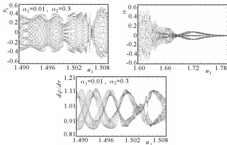
Fig. 4. Bifurcation diagrams for  $y_1$ ,  $\alpha$  and  $d\varphi/d\tau$  in the region  $u_1 \in (1.49, 1.51)$  for:  $u_2 = 1.5$ ,  $q = 0.2$ ,  $\beta = 0.5$ ,  $a_1 = 0.01$ ,  $a_2 = 0.3$ ,  $\gamma_1 = 0.001$ ,  $\gamma_2 = \gamma_3 = \gamma_4 = 0$
