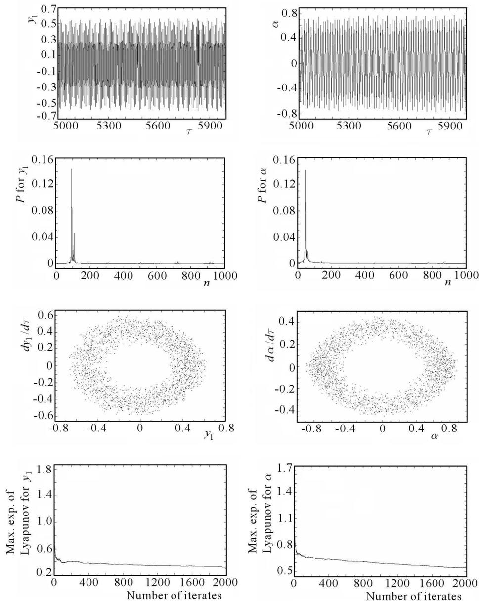
Fig. 5. Time histories, power spectral densities, Poincaré's maps and maximum Lyapunov exponents corresponding to coordinates  $y_1$  and  $\alpha$  for the control parameter  $u_1 = 1.499$  and for:  $u_2 = 1.5$ ,  $q = 0.2$ ,  $\beta = 0.5$ ,  $a_1 = 0.01$ ,  $a_2 = 0.3$ ,  $\gamma_1 = 0.001$ ,  $\gamma_2 = \gamma_3 = \gamma_4 = 0$
