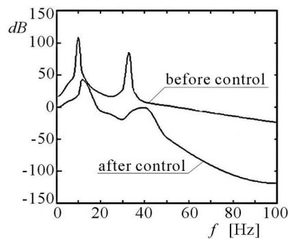
Fig. 3. Comparison of the acceleration level of the middle mass block
