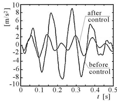
Fig. 4. Comparison of the acceleration response of the middle mass block
