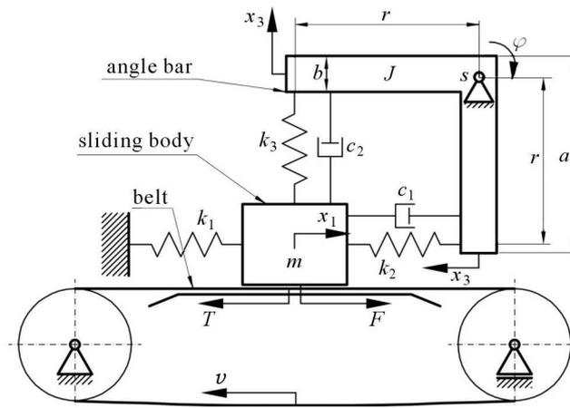
Fig. 1. The analysed 2-DOF system
