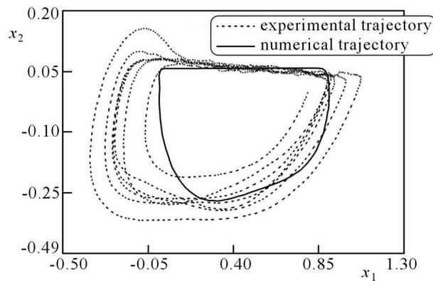
Fig. 4. Similarity of the experimental and numerical phase trajectories of the block for  $T_-$  friction characteristic
