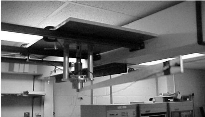
Fig. 2. Experimental set-up of the slewing flexible beam-like structure (Fenili, 2000; Fenili *et al.*, 2001)
