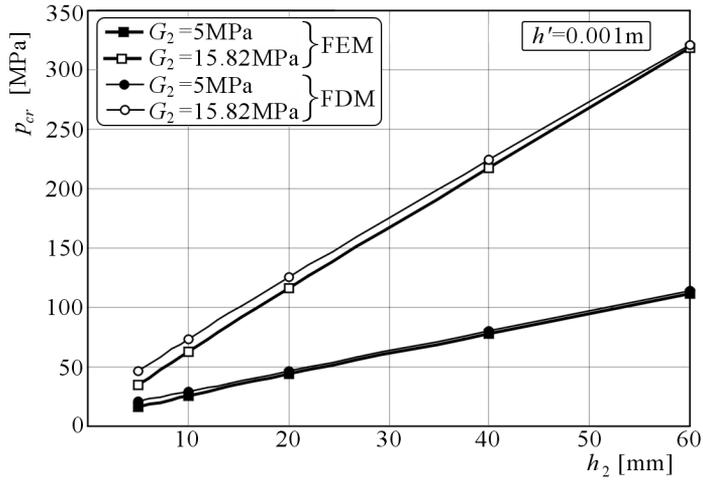
Fig. 15. Critical load distribution depending on the core for the plate with equal layer deflections, loaded on the outer perimeter and with facing thickness  $h' = 0.001$  m
