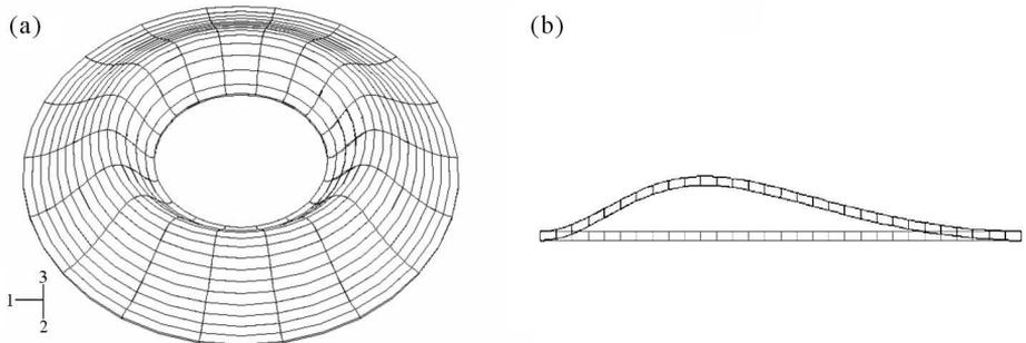
Fig. 19. Axially-symmetric buckling form of the plate compressed on the inner edge: (a) full annulus model, (b) model built of axisymmetric elements
