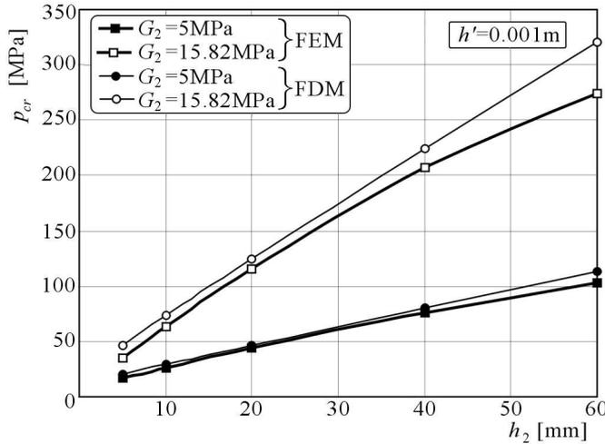
Fig. 8. Critical static load distribution depending on the core for the plate loaded on the outer perimeter with facing thickness  $h' = 0.001$  m
