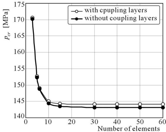
Fig. 20. Convergence of critical loads
