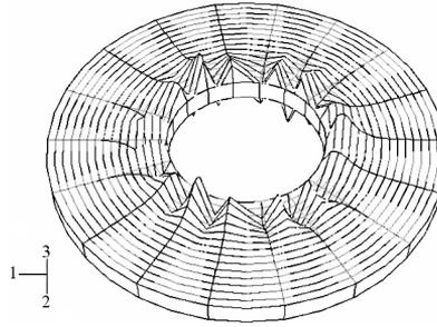
Fig. 11. Critical buckling form of the plate with parameters:  $h' = 0.0005$  m,  $h_2 = 0.06$  m and  $G_2 = 15.82$  MPa, loaded on outer perimeter
