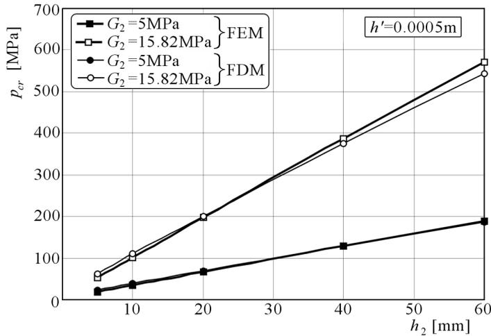
Fig. 14. Critical load distribution depending on the core for the plate with equal layer deflections, loaded on the outer perimeter and with facing thickness  $h' = 0.0005$  m
