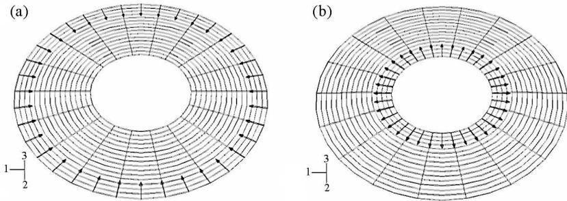
Fig. 2. Scheme of the plate loaded: (a) on the outer perimeter, (b) on the inner perimeter
