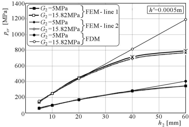
Fig. 9. Critical static load distribution depending on the core for the plate loaded on the inner perimeter with facing thickness  $h' = 0.0005$  m
