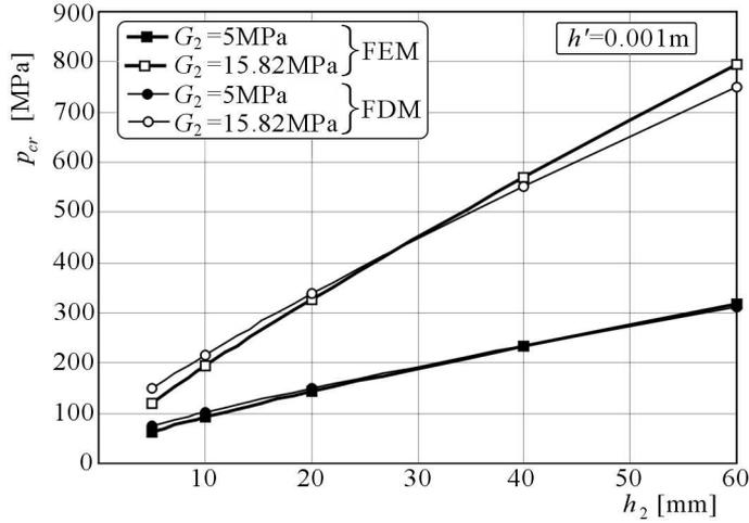
Fig. 17. Critical load distribution depending on the core for the plate with equal layer deflections, loaded on the inner perimeter and with facing thickness  $h' = 0.001$  m
