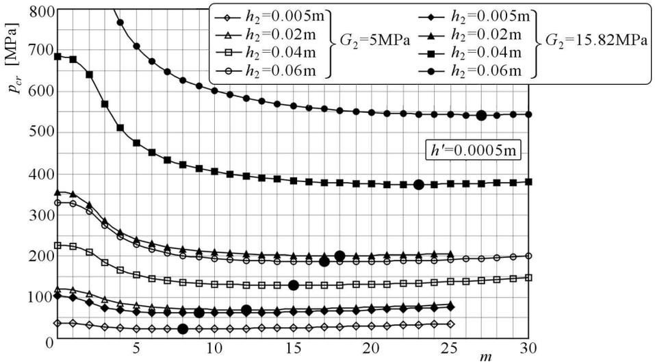
Fig. 3. Critical static load distributions depending on the number of buckling waves for the plate compressed on the outer perimeter with facing thickness  $h' = 0.0005\text{m}$
