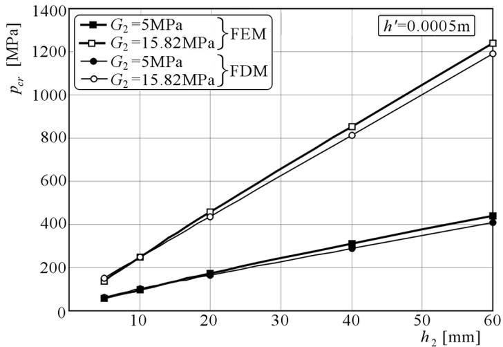
Fig. 16. Critical load distribution depending on the core for the plate with equal layer deflections, loaded on the inner perimeter and with facing thickness  $h' = 0.0005$  m
