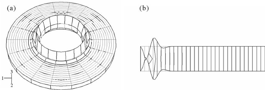
Fig. 12. Critical buckling form of the plate with parameters:  $h' = 0.0005$  m,  $h_2 = 0.06$  m and  $G_2 = 15.82$  MPa, loaded on inner perimeter and built: (a) as full annulus, (b) of axisymmetric elements
