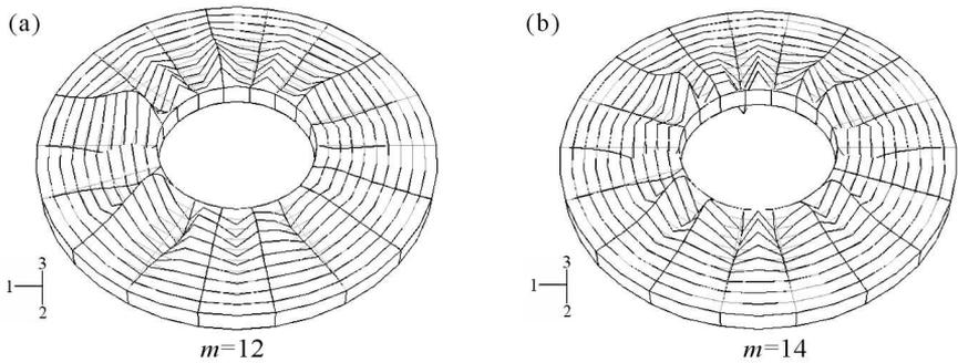
Fig. 18. Critical buckling form of the plate loaded on the outer perimeter with equal layer deflections and with parameters  $h' = 0.0005$  m,  $h_2 = 0.06$  m: (a)  $G_2 = 5$  MPa, (b)  $G_2 = 15.82$  MPa
