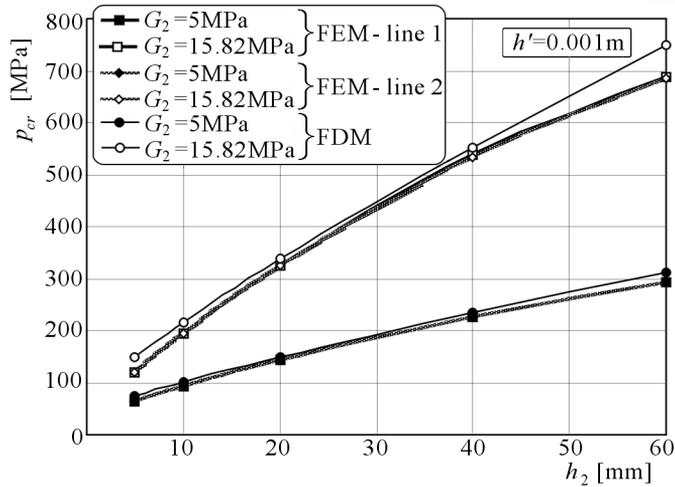
Fig. 10. Critical static load distribution depending on the core for the plate loaded on the inner perimeter with facing thickness  $h' = 0.001$  m
