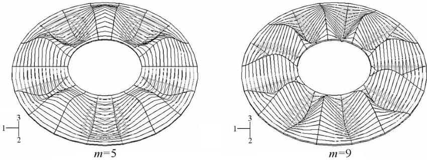
Fig. 13. Exemplary critical buckling forms of plates loaded on the outer perimeters
