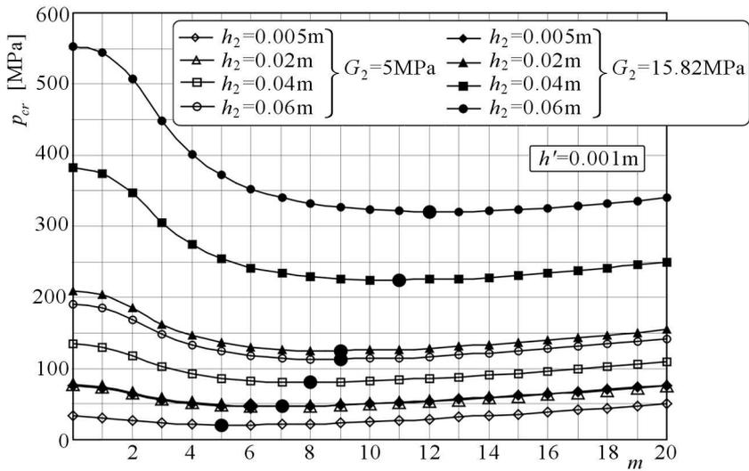
Fig. 4. Critical static load distributions depending on the number of buckling waves for the plate compressed on the outer perimeter with facing thickness  $h' = 0.001\text{m}$
