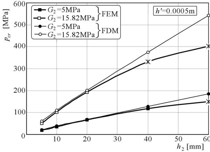
Fig. 7. Critical static load distribution depending on the core for the plate loaded on the outer perimeter with facing thickness  $h' = 0.0005$  m
