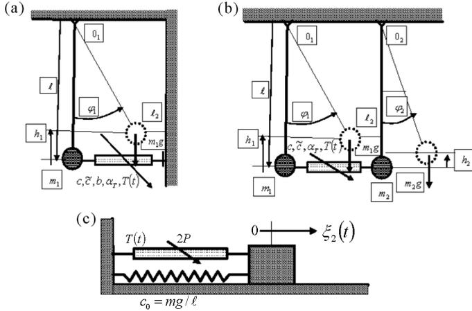
Fig. 7. (a) System with one pendulum coupled by the standard light visco-thermoelastic element. (b) System with two pendula intercoupled by the standard light thermorheological element. (c) Thermo-rheological system; partial oscillator 2
