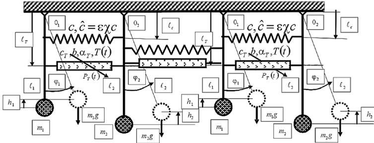
Fig. 1. System with four pendula interconnected by standard light thermo-modified hereditary element and nonlinear springs
