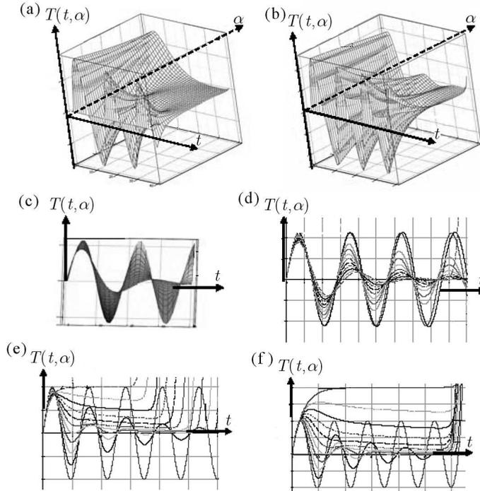
Fig. 5. Time function surfaces of  $\tilde{T}_1(t, \alpha)$ , (6.12)<sub>2</sub>, for different kinetic and creep parameters of the-one pendulum system; (a) for  $\omega_{0\alpha}^2/(\tilde{\omega}_0^2 + \omega_{00}^2) = 1$ , (b) for  $\omega_{0\alpha}^2/(\tilde{\omega}_0^2 + \omega_{00}^2) = 1/16$ , (c) for  $\omega_{0\alpha}^2/(\tilde{\omega}_0^2 + \omega_{00}^2) = 1/9$ . (d) for  $\omega_{0\alpha}^2/(\tilde{\omega}_0^2 + \omega_{00}^2) = 9$
