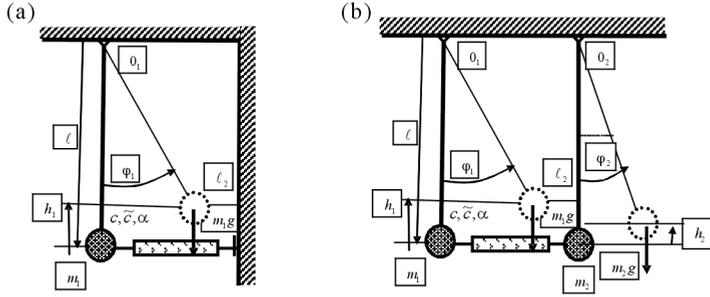
Fig. 3. System with one pendulum coupled (a) and with two pendula intercoupled (b) by standard light creep element
