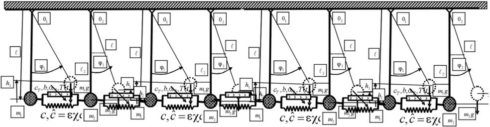
Fig. 2. System with "chain" pendula interconnected by standard light thermo-modified hereditary elements and creep elements
