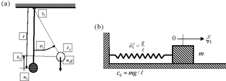
Fig. 6. (a) System with one free pendulum. (b) Thermo-rheological system; partial oscillator 1
