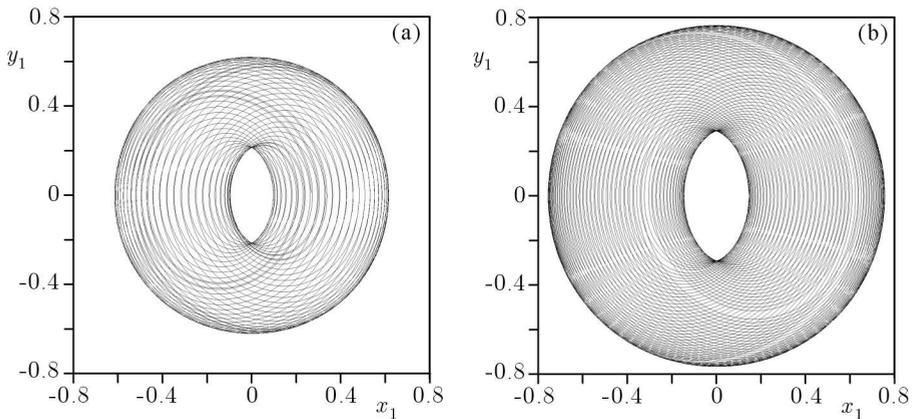
Fig. 8. Quasi periodic tori projected on the physical master coordinates  $x_1, y_1$  obtained from the original system (a), and after superposition of motion of modal oscillators (b); model with two self-excitation terms (variant II, (4.2))
