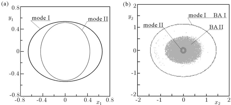
Fig. 2. Phase plane  $x_1y_1$  with limit cycles (a) and basins of attraction in the phase plane  $x_2y_2$  (b) for the first and second vibration modes; model with one self-excitation term (variant I, (4.1))
