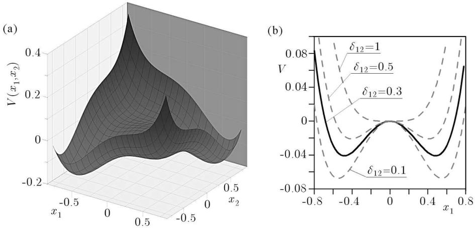
Fig. 9. Potential surface versus system physical coordinates (a) and the cross-section for  $x_2 = 0$  (b)
