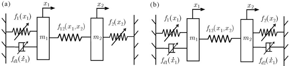
Fig. 1. Physical model of the system with one (a) and two (b) nonlinear dampers
