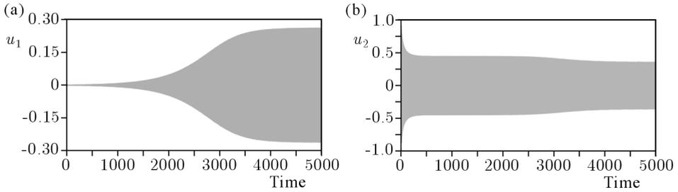
Fig. 7. Time histories in normal coordinates obtained for the first (a) and the second (b) vibration modes, model with two self-excitation terms (variant II, (4.2)), long time after activation
