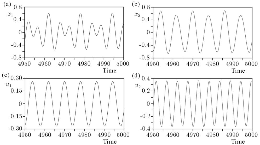
Fig. 4. Time histories in physical coordinates (a), (b) and normal coordinates obtained for the first (c) and the second (d) vibration mode; model composed of two self-excitation terms (variant II, (4.2))
