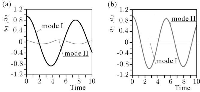
Fig. 6. Time histories in normal coordinates obtained for the first (a) and the second (b) vibration mode; model with two self-excitation terms (variant II, (4.2)), short time after activation
