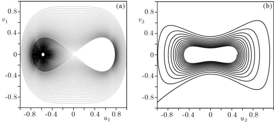
Fig. 13. Modal response of the system for  $\delta_{12} = 0.6$ ; (a) numerical solution of Eq. (5.3) and (b) Eq. (5.4)
