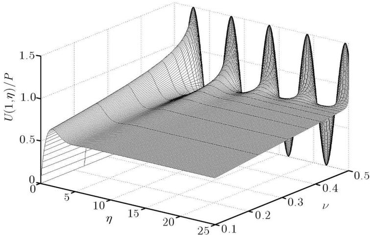
Fig. 3. Calculated relative displacement of the cavity surface  $U(1, \eta)/P$  versus dimensionless time  $\eta$  and Poisson's ratio  $\nu$
