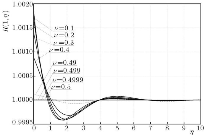
Fig. 5. Calculated relative density  $R$  versus dimensionless time  $\eta$  for  $\xi = 1$  and selected values of Poisson's ratio  $\nu$
