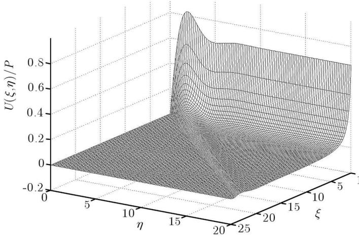
Fig. 4. Calculated relative displacement  $U(\xi, \eta)/P$  versus dimensionless variables  $\xi$  and  $\eta$  for Poisson's ratio  $\nu = 0.3$
