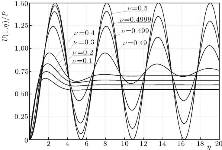
Fig. 2. Calculated relative displacement of the cavity surface  $U(1, \eta)/P$  versus dimensionless time  $\eta$  for selected values of Poisson's ratio  $\nu$
