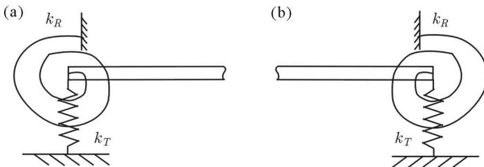
Fig. 1. General boundary conditions of the beam (a) at  $x = 0$  (b) at  $x = l$
