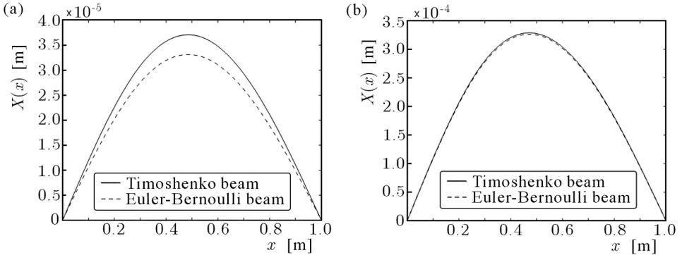
Fig. 2. Vibration amplitudes of the simply supported beam (a) stocky beam (b) slender beam
