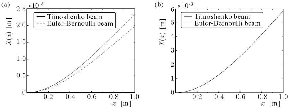
Fig. 3. Vibration amplitudes of the cantilever beam (a) stocky beam (b) slender beam
