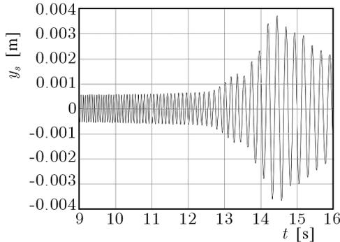
Fig. 7. Graph of the machine body mass centre displacement  $y_s$  during the run-down phase. Experiment
