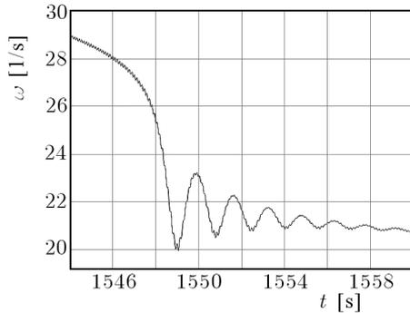
Fig. 8. Graph for vibrator angular velocity during run-down phase in the area of resonant frequency. Computer simulation
