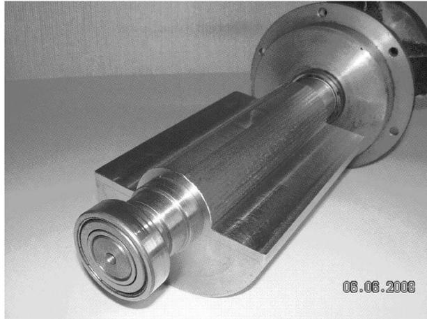
Fig. 5. Inertia vibrator used for the purpose of experiment
