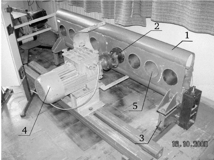
Fig. 4. Test Stand. 1 – machine body, 2 – inertia vibrator, 3 – spiral spring, 4 – electric motor, 5 – hole for an additional mass
