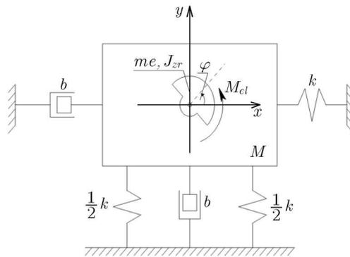
Fig. 1. Model of a vibratory machine
