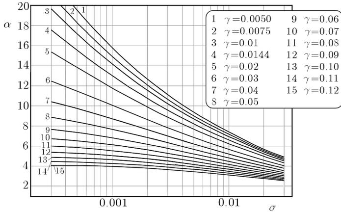
Fig. 3. Multiplication factor  $\alpha$  of the machine body vibration amplitude for the run-down phase;  $\alpha = A_{max}/A_u$ , where  $A_{max}$  – resonance amplitude
