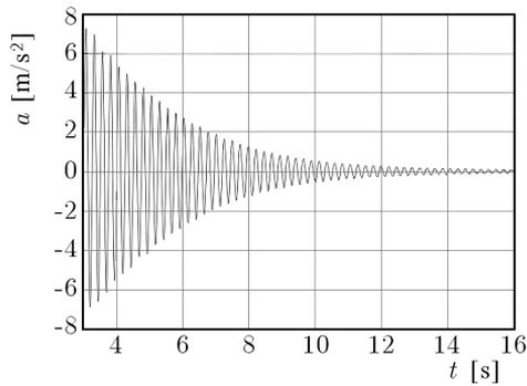
Fig. 6. Graph showing natural vibration acceleration of the machine body recorded during the experiment
