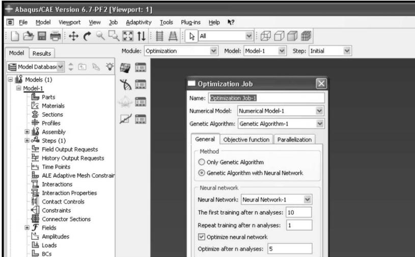
Fig. 7. Optimization module for Abaqus/CAE
