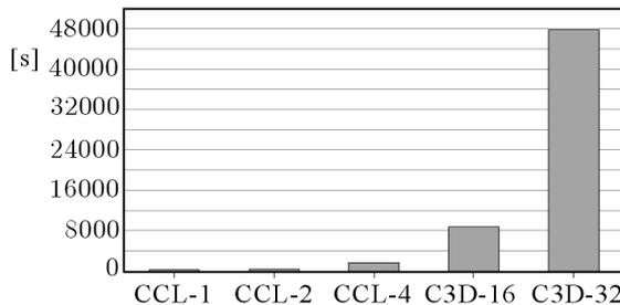
Fig. 3. The Wallclock time for 3D analyses with the use of cylindrical (CCL-x) and 3D solid elements (C3D-x)
