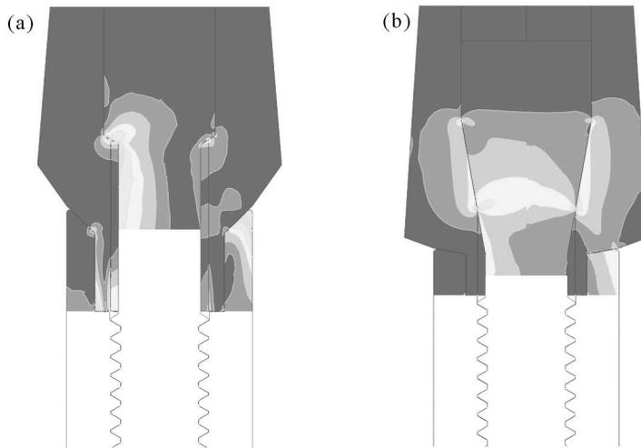
Fig. 14. Mises stress in the initial (a) and final (b) dental implant
