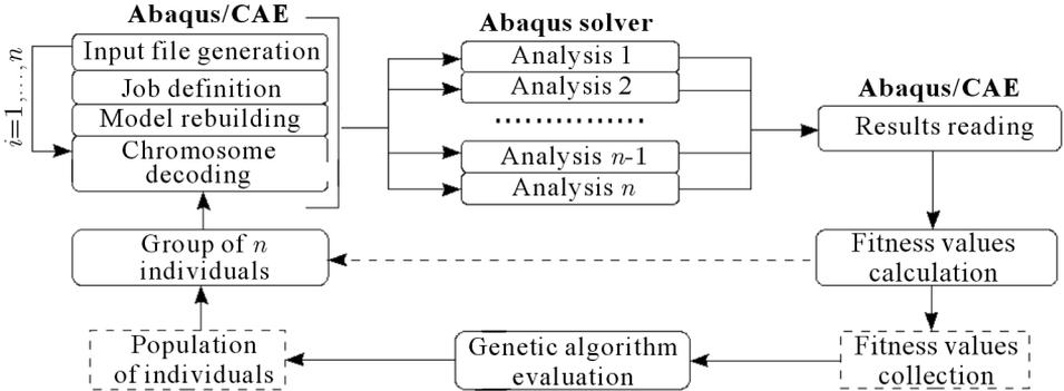
Fig. 9. Scheme of genetic algorithm evaluation processing
