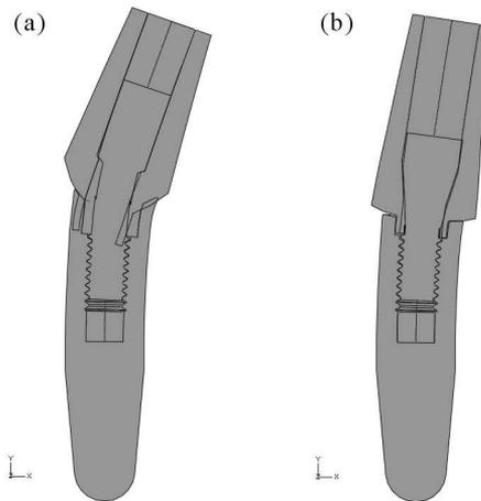
Fig. 13. Deformation of the initial (a) and final (b) dental implant (displacement scaled up 40 times)
