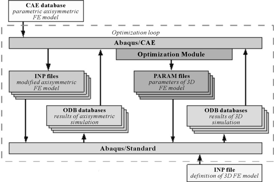
Fig. 10. The procedure of building of an FE implant model during the optimization process
