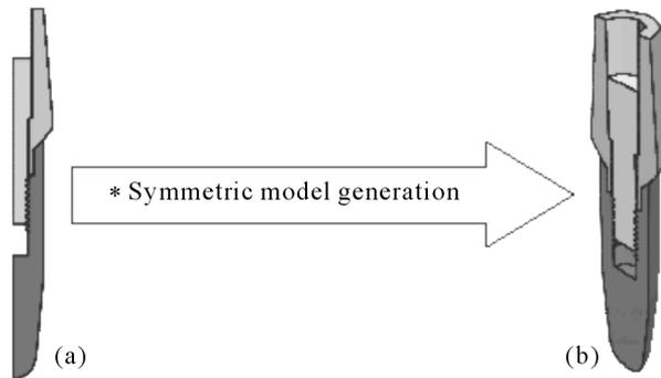
Fig. 2. Numerical models of the implant: axisymmetric (a) and 3D (b)
