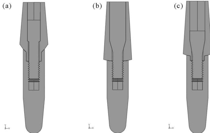
Fig. 12. Initial (a) and new (b, c) shapes of dental implant
