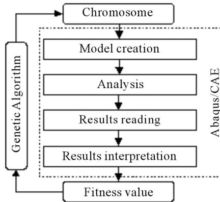
Fig. 8. Individual evaluation procedure
