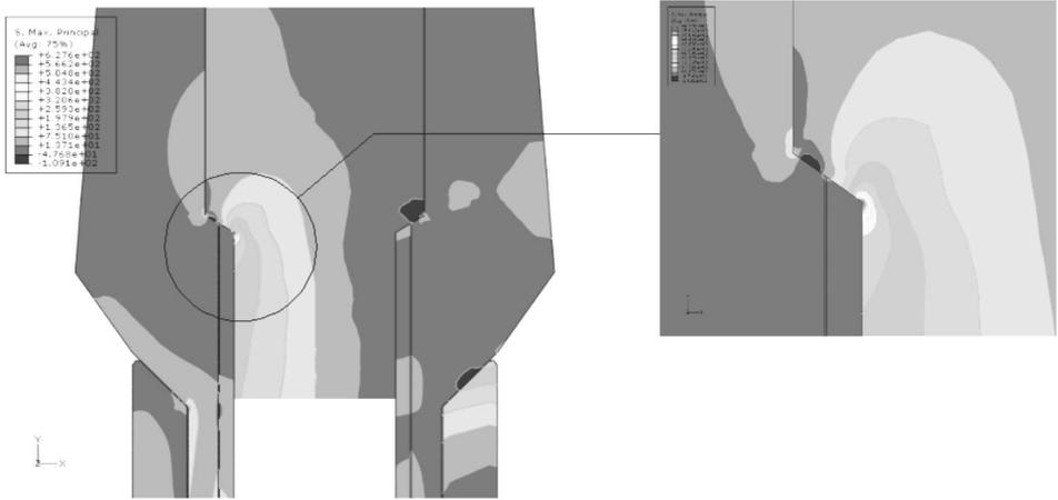
Fig. 5. Huber-Mises stress in the initial design of a dental implant
