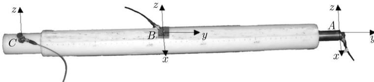
Fig. 7. A view of the accelerometers location
