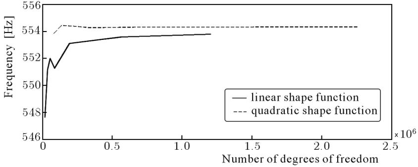
Fig. 4. Convergence of the first eigenfrequency for APB system
