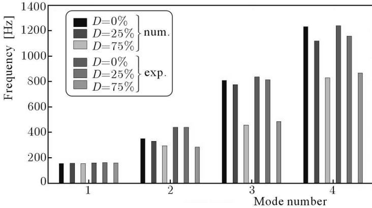
Fig. 9. A comparison of numerical and experimental results for PB system
