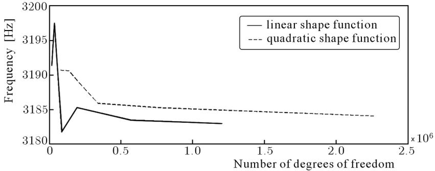
Fig. 5. Convergence of the fourth eigenfrequency for APB system
