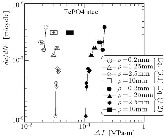
Fig. 3. Fatigue crack growth rate  $da/dN$  versus the  $\Delta J$  parameter with and without the factor  $K_t$
