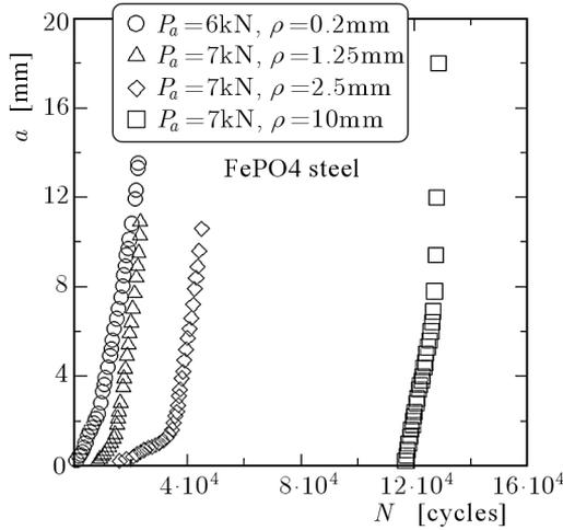
Fig. 2. Fatigue crack length versus number of cycles for different radii of the notch root
