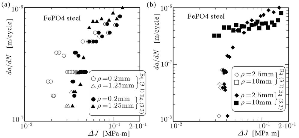
Fig. 4. Fatigue crack growth rate  $da/dN$  versus the  $\Delta J$  parameter with and without the correction factor  $Y_2$  for (a)  $\rho = 0.2, 1.25$  mm and (b)  $\rho = 2.5, 10$  mm
