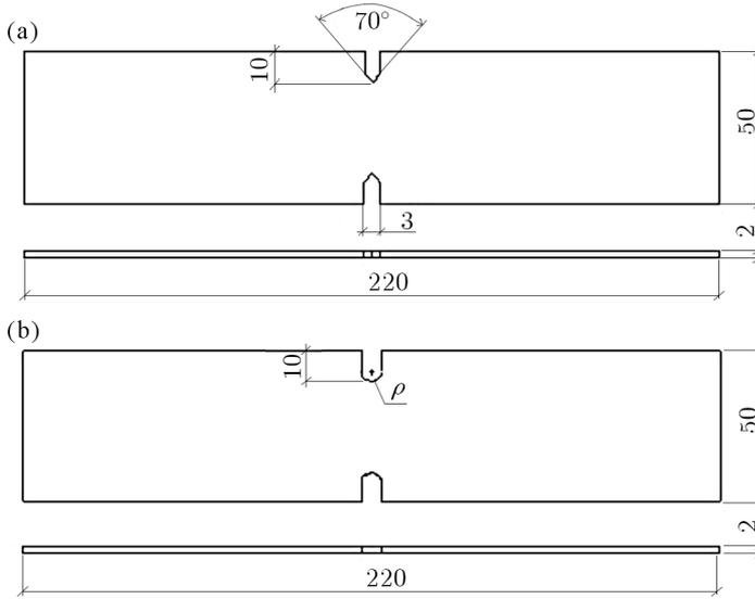
Fig. 1. Geometry of specimens characterised by: (a) sharp and (b) blunt notches; all dimensions in mm
