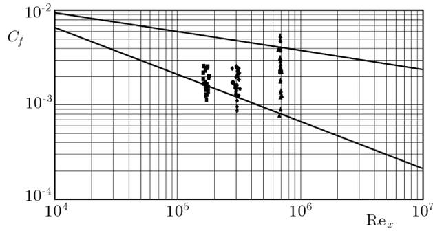
Fig. 10. Local friction coefficient  $C_f = f(\tau)$  for  $Re_x = 168843, 298640$  and  $686918$
