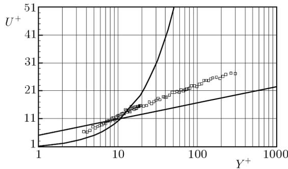
Fig. 7. Temporary velocity profile for  $Re = 168843$  and  $\tau = 0.06$
