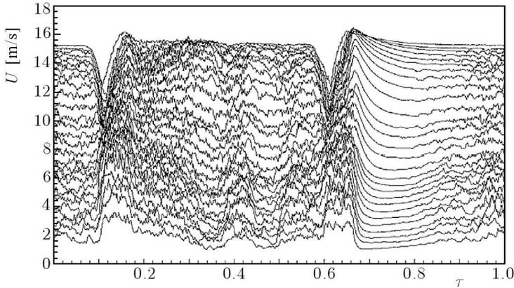
Fig. 5. Phase averaged time traces of velocity,  $Re_x = 33414$
