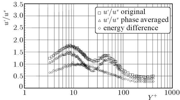
Fig. 11. Distribution of velocity fluctuations for:  $Re_x = 168853$ : time and phase averaged and turbulent
