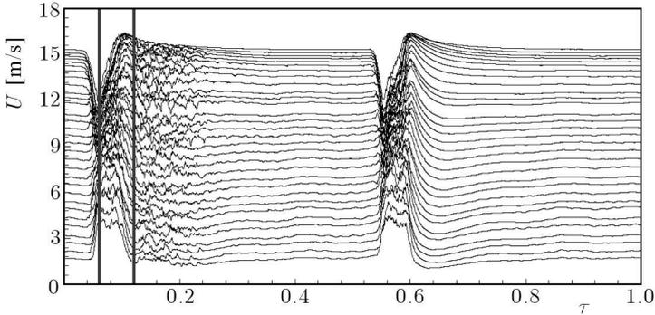
Fig. 4. Phase averaged time traces of velocity,  $Re_x = 168853$
