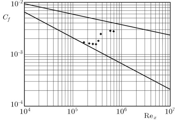
Fig. 3. Distribution of the local shear stress coefficient  $C_f$  versus  $Re_x$ .
