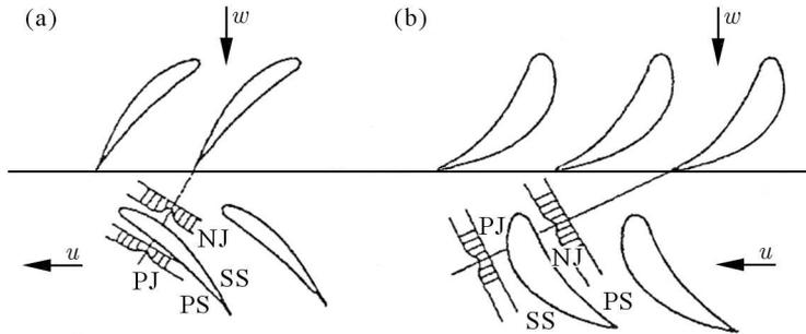
Fig. 1. Positive and negative jets of wakes in a compressor (a) and in a turbine stage (b) (Wierciński, 1999)
