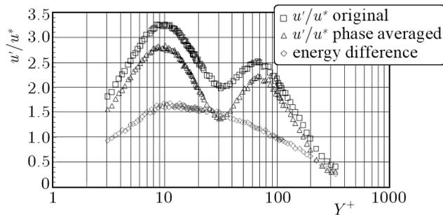
Fig. 12. Distribution of velocity fluctuations for:  $Re_x = 686918$ : time and phase averaged and turbulent
