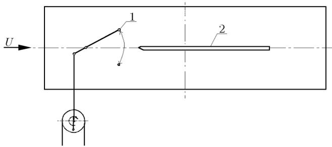
Fig. 2. Experimental stand, 1 – rod in motion as a wake generator, 2 – plate
