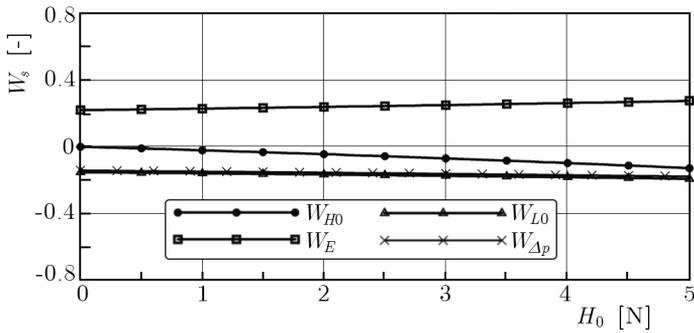
Fig. 11. Relative sensitivity coefficients calculated for M3 model vs. initial junction force  $H_0$
