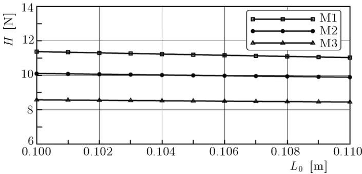
Fig. 6. Junction force  $H$  in M1, M2, M3 models vs. initial cable length  $L_0$
