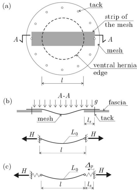
Fig. 2. Mathematical model of the fascia-mesh system; (a) scheme of the fascia-mesh junction with one strip distinguished for further cable model, (b) cable model with stiff supports, (c) cable with support springs representing an elastic mesh in the support zone as well as with displacements of cable edges related to the flexible edges of the hernia
