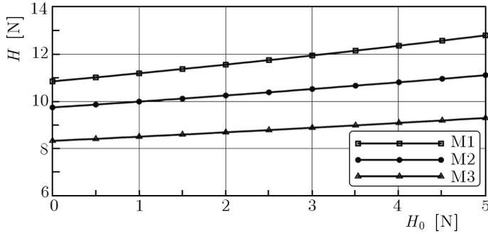
Fig. 7. Junction force  $H$  in M1, M2, M3 models vs. initial junction force  $H_0$
