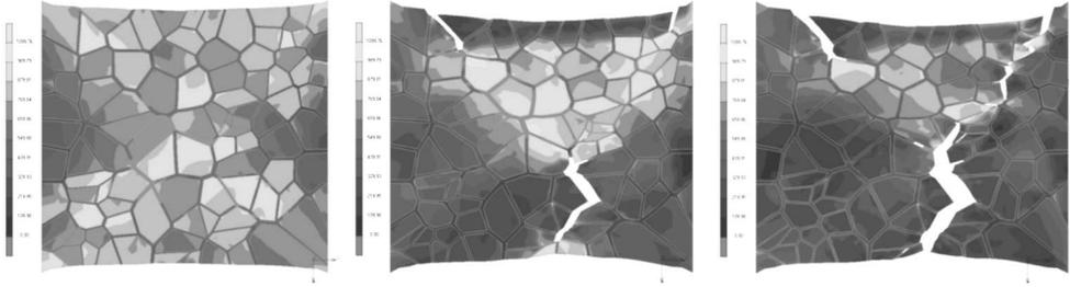
Fig. 16. Stress distribution in simulation of tension of grain structure
