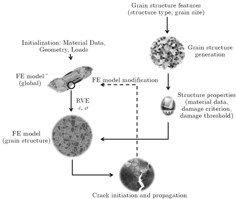
Fig. 13. Idea of multiscale ductile damage model
