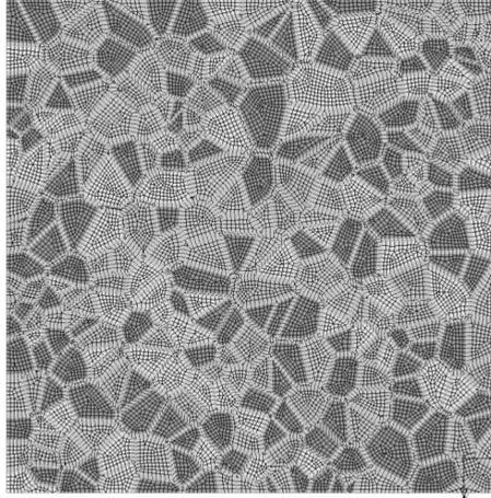
Fig. 14. Exemplary FEM model of the structure with 300 grains with grain boundaries (applied material data)
