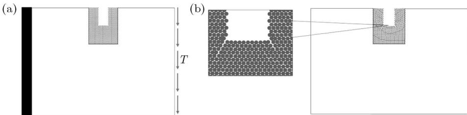
Fig. 1. Exemplary concurrent multiscale model (Madej *et al.*, 2008). (a) Notched cantilever beam subjected to end load. Vicinity of the notch modelled at atomic scale. (b) Simulation result. Cracks initiation in the corners of the notch
