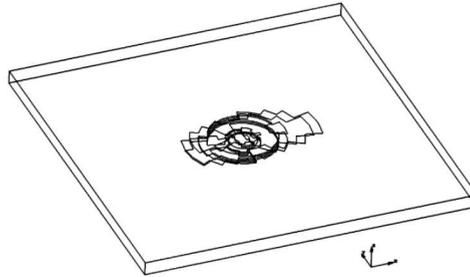
Fig. 6. Laminate plate with delamination
