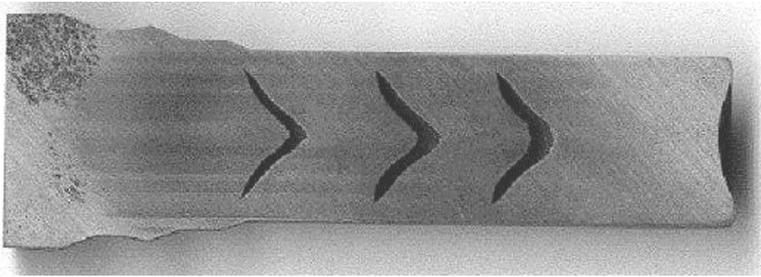
Fig. 10. Chevron cracks during drawing process (MSC.Marc Mentat, 2008)
