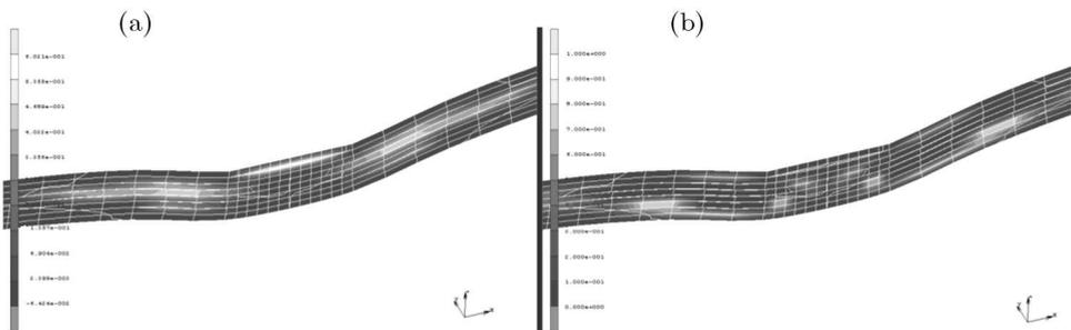
Fig. 5. Distribution of damage index (a), and delamination index (b)
