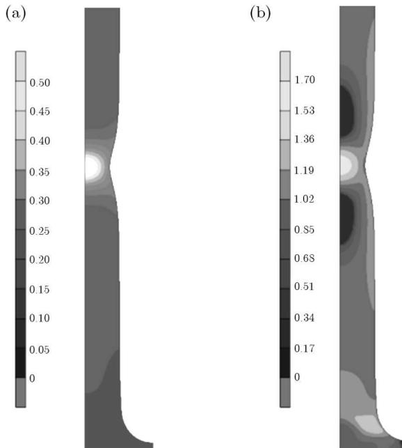
Fig. 9. Oyane (a) and Principal Stress (b) damage indicators during virtual tension test
