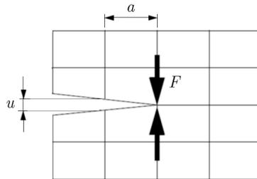
Fig. 4. Model employed for VCCT method (MSC.Marc Mentat, 2008)
