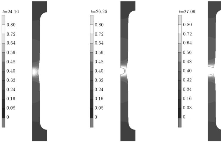
Fig. 8. Subsequent stages of tensile test
