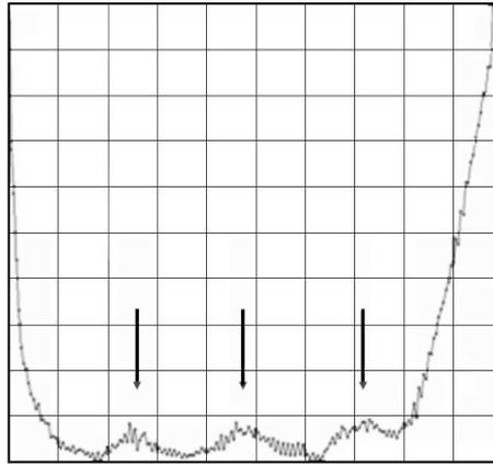
Fig. 12. Force diagram for drawing process with significant force drops related to ductile fracture
