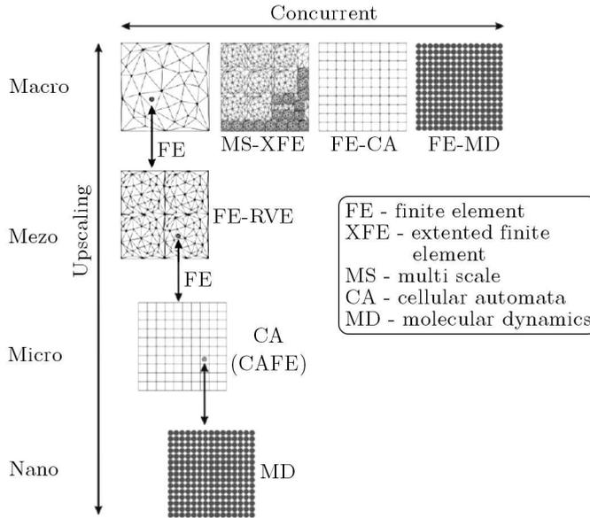
Fig. 2. Classification of multiscale modelling methods Madej *et al.*, 2008
