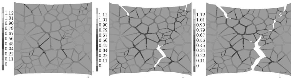
Fig. 15. Damage indicator distribution in simulation of tension of grain structure
