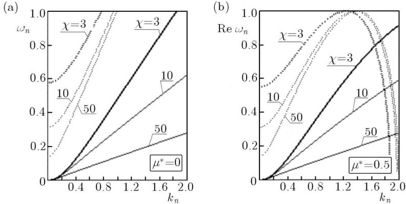
Fig. 3. Natural frequency vs. wave number  $k_n$  for the Timoshenko beam at three values of shear parameter  $\chi$  (a) elastic material; (b) visco-elastic material (solid curves – the first branch, dotted curves – the second one)
