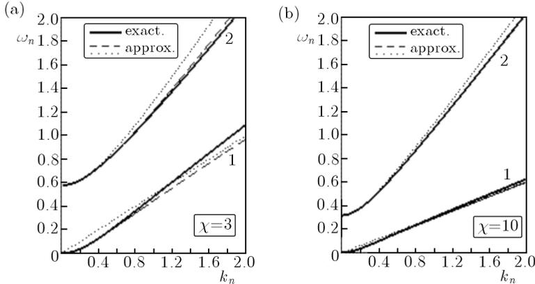
Fig. 2. Natural frequency vs. wave number  $k_n$  for the elastic Timoshenko beam at  $\chi = 3$  (a) and  $\chi = 10$  (b). 1, 2 – the first and second frequency spectrum, solid curves – exact solution, dashed and dotted lines – approximate solutions by (3.15), (3.16) and (3.19), (3.20), respectively
