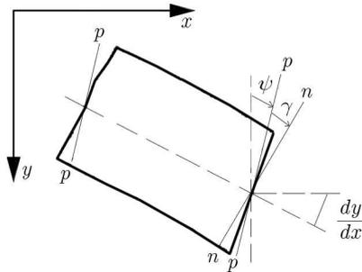
Fig. 1. Element of the beam and scheme of deformation of the beam flat cross section;  $n$ - $n$  is the normal plane (to the bent axis),  $p$ - $p$  is the tangent plane to the deformed cross section (at the neutral axis)
