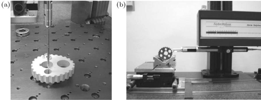
Fig. 8. Measurement of geometrical features (a) and roughness features (b) of noncircular wheels executed in LEDM
