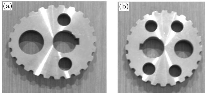
Fig. 6. Wheels of the variable speed transmission system: (a) noncircular wheel, (b) circular eccentrically mounted wheel
