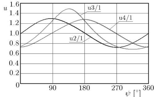
Fig. 9. Changes in the transmission ratio of: wheel 2 in relation to wheel 1 ( $u_{2/1}$ ), wheel 3 in relation to wheel 1 ( $u_{3/1}$ ), wheel 4 in relation to wheel 1 ( $u_{4/1}$ ). Along the horizontal axis there are marked values of the angle ( $\psi$ , measured in degrees) of rotation of the driving wheel
