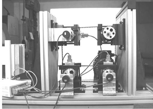
Fig. 5. Four-wheel transmission systems installed in LEDM (Laboratory for Experimental Design and Manufacturing at the Faculty of Machines and Transport, Poznan University of Technology); the system has two circular wheels, one noncircular wheel and one eccentrically mounted wheel
