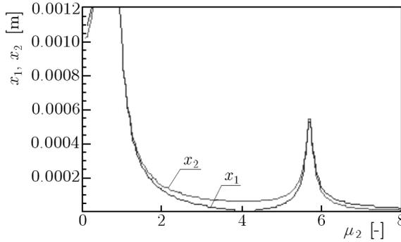
Fig. 3. Displacements  $x_1$  and  $x_2$  of the considered masses presented in functions of the frequency ratio  $\mu_2$
