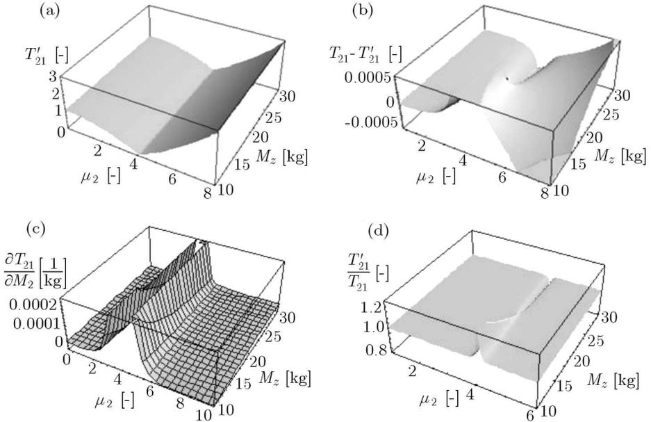
Fig. 6. Amplitude-frequency characteristic of: (a) transfer function  $T'_{21}$ , (b)  $T'_{21} - T_{21}$ , (c) derivative  $\partial T_{21} / \partial M_2$ , (d)  $T'_{21} / T_{21}$  in the function of mass ( $M_2 + \Delta M_2$ ) and  $\mu_2$  (values obtained for  $\Delta M_2 \in \langle -10, +10 \rangle$ ), where  $M_z = M_2 + \Delta M_2$  kg
