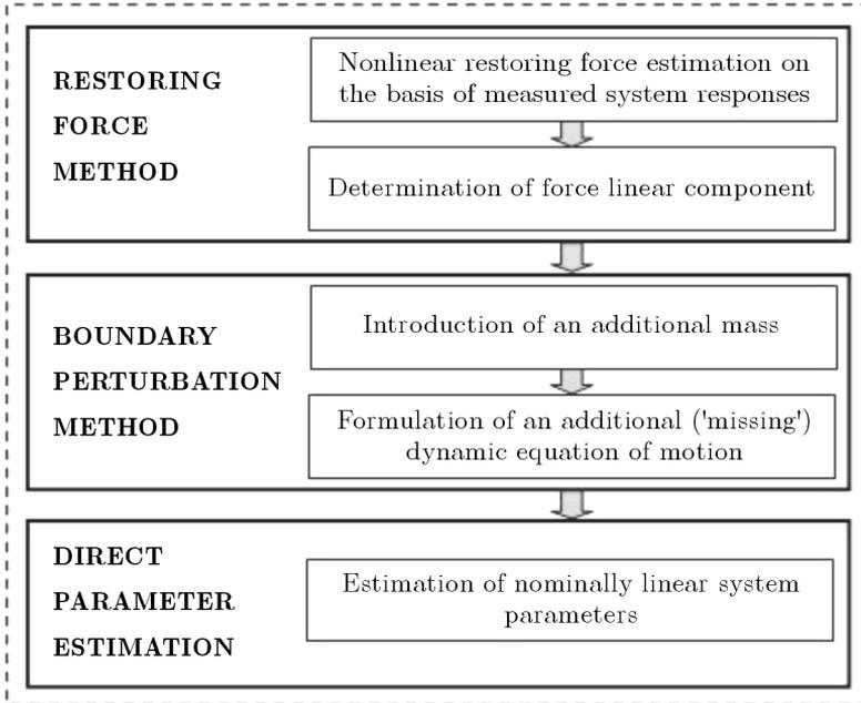
Fig. 1. Proposed and verified (Iwaniec, 2009b) identification method of nonlinear systems working under operational loads
