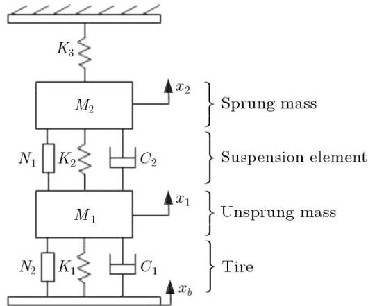
Fig. 2. Discrete model of a 2 degree-of-freedom nonlinear system (vehicle suspension system)
