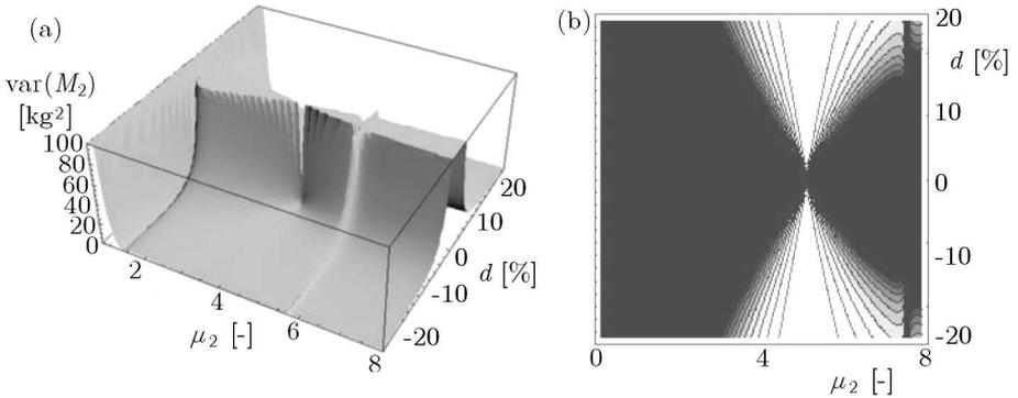
Fig. 10. Variance of mass  $M_2$  in function of  $d$  and  $\mu_2$ , (a) three-dimensional function shape, (b) isometric projection on the plane  $d, \mu_2$
