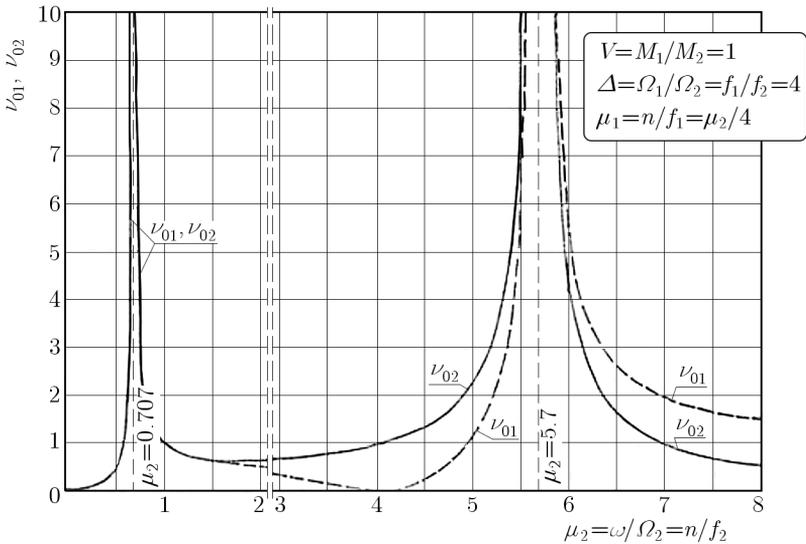
Fig. 4. Amplitude-frequency characteristics of displacements of two-degree-of-freedom system in function of  $\mu_2$  (with the influence of damping neglected) (Goliński, 1979)
