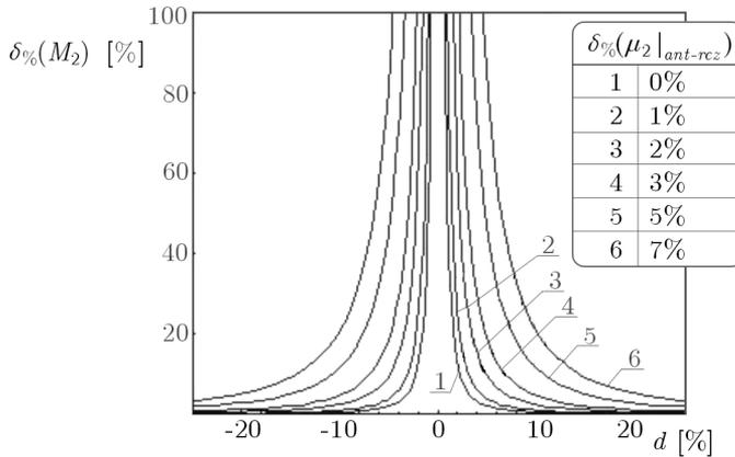
Fig. 11. Relative error of the mass  $M_2$  estimated on the basis of change in the system response resulting from addition or subtraction of the mass  $\Delta M_2$  in the range of  $d = \pm 25\%$
