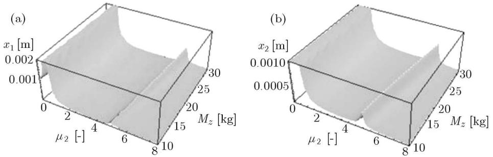
Fig. 5. Amplitude-frequency characteristic of displacements of mass (a)  $M_1$  and (b)  $M_2$  in function of  $\mu_2$  and the mass value  $(M_2 + \Delta M_2)$ ,  $\Delta M_2 \in \langle -10, +10 \rangle$ , where  $M_z = M_2 + \Delta M_2$  kg
