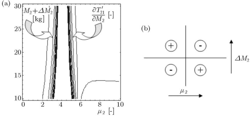
Fig. 7. Sensitivity  $\partial T'_{21}/\partial M_2$  of the transfer function to changes in mass  $M_2$  – arrows determine the direction of increase in the derivative (a), monotonicity of the function determining the mass  $M_2$  in the neighborhood of frequency corresponding to the minimum of transfer function and additional mass (b)
