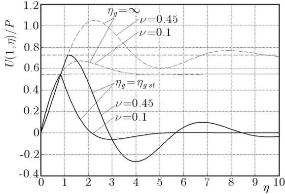
Fig. 7. Variation of the displacement ( $U/P$ ) of the cavity wall ( $\xi = 1$ ) loaded by the finite time pressure pulse versus  $\eta$  for  $\eta_g = \eta_{gst}$  and selected values of  $\nu$
