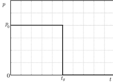
Fig. 2. Scheme of the finite pulse of constant pressure
