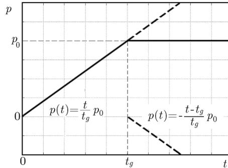
Fig. 3. Schematic variation of quasi-static pressure in time
