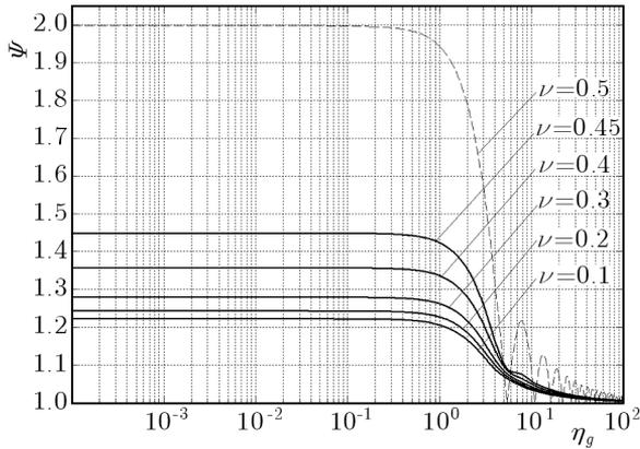
Fig. 6. Variation of the dynamic coefficient of load  $\Psi$  on the cavity wall ( $\xi = 1$ ) loaded by quasi-static pressure versus  $\eta_g$  for selected values of  $\nu$
