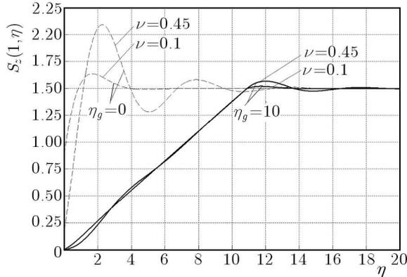
Fig. 5. Variation of the reduced stress  $S_z$  on the cavity wall ( $\xi = 1$ ) loaded by quasi-static pressure versus  $\eta$  for  $\eta_g = 10$  and selected values of  $\nu$
