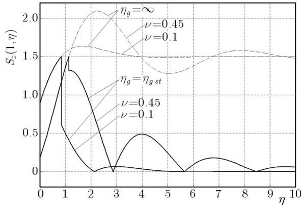
Fig. 8. Variation of the reduced stress  $S_z$  on the cavity wall ( $\xi = 1$ ) loaded by the finite time pressure pulse versus  $\eta$  for  $\eta_g = \eta_{g\ st}$  and selected values of  $\nu$
