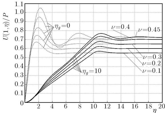
Fig. 4. Variation of the displacement ( $U/P$ ) of the cavity wall ( $\xi = 1$ ) loaded by quasi-static pressure versus  $\eta$  for  $\eta_g = 10$  and selected values of  $\nu$
