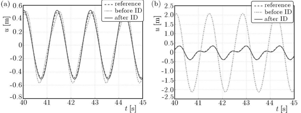
Fig. 9. Case 5. Time history at different degrees of freedom; (a) DOF 2 – not control point, (b) DOF 11 – control point
