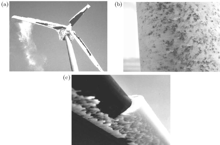
Fig. 1. Examples of the effect of ice and bugs on wind-turbine and rotorcraft blades; (a) ice on wind turbine, (b) bugs on wind turbine, (c) ice on helicopter blade
