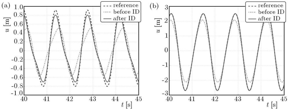
Fig. 11. Case 6. Time history at different degrees of freedom; (a) DOF 2 – not control point, (b) DOF 11 – control point
