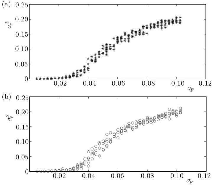
Fig. 5. The variance of the generated voltage,  $\sigma_v$ , for different noise distributions (a) Gaussian and (b) uniform
