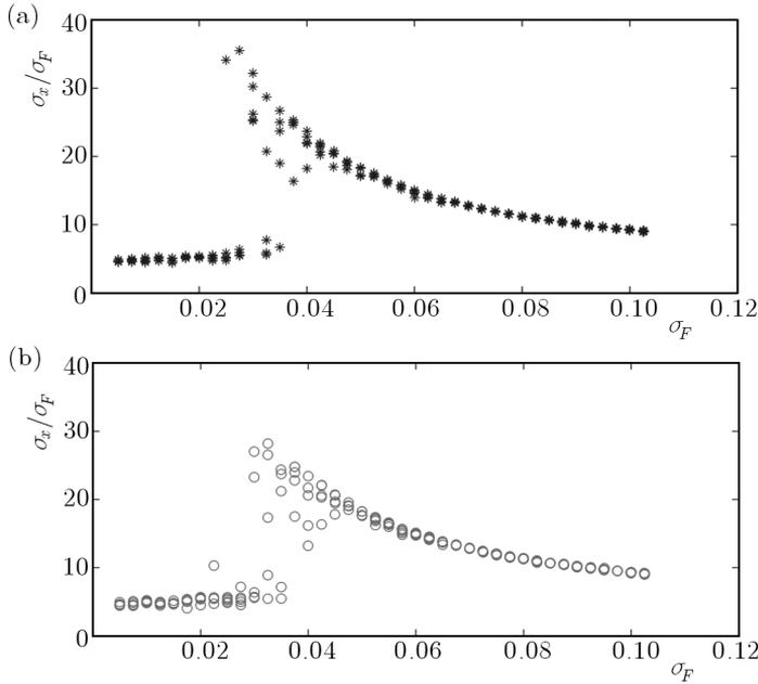
Fig. 2. The displacement signal to noise ratio  $\sigma_x/\sigma_F$  versus noise intensity  $\sigma_F$ , where  $\sigma_x$  is the standard deviation of the beam displacement and  $\sigma_F$  is the standard deviation of the noise excitation for different noise distributions (a) Gaussian and (b) uniform
