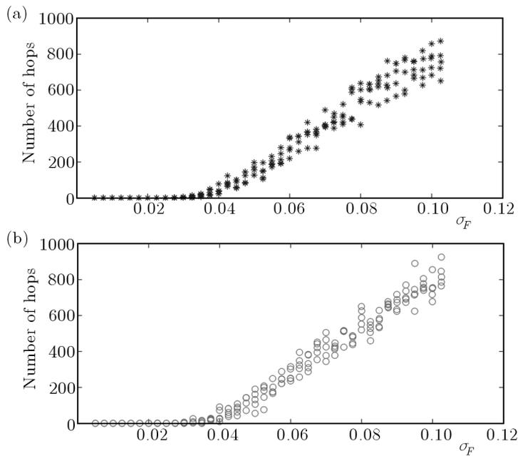
Fig. 4. The number of hops between potential wells for different noise distributions (during the investigated simulation interval) (a) Gaussian and (b) uniform
