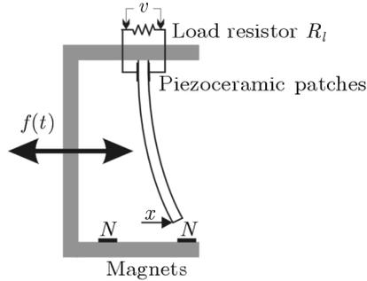
Fig. 1. Schematic of the piezomagnetoelastic device (Litak *et al.*, 2010)
