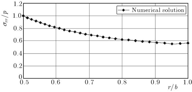
Fig. 7. Variation of the distribution of radial compressive stress
