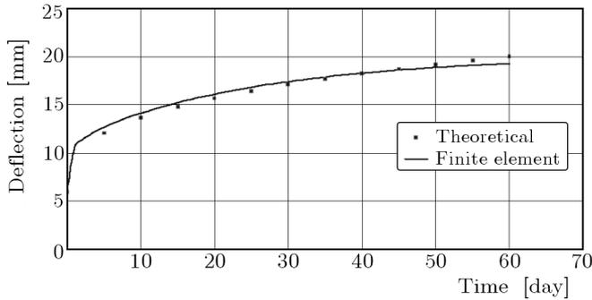
**Fig. 2.** Deflection in viscoelastic panel versus time
