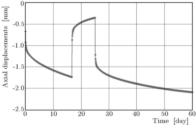
Fig. 4. Axial displacement in viscoelastic panel versus time
