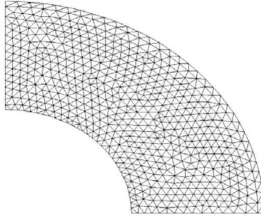
Fig. 6. Viscoelastic cylinder under internal pressure: finite element mesh
