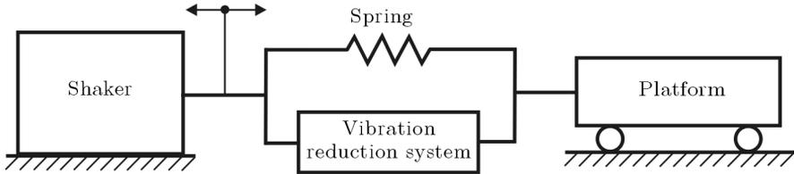
Fig. 1. Simplified mechanical structure of the stand
