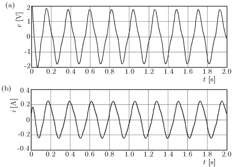
Fig. 5. Time histories of: (a) electromotive force  $e$ , (b) current  $i$  in the generator-MR damper circuit
