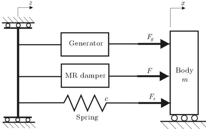
Fig. 2. Schematic diagram of the mechanical sub-system
