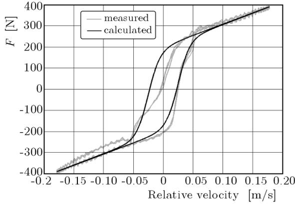
Fig. 4. Damper force  $F$  versus relative velocity  $\dot{z} - \dot{x}$
