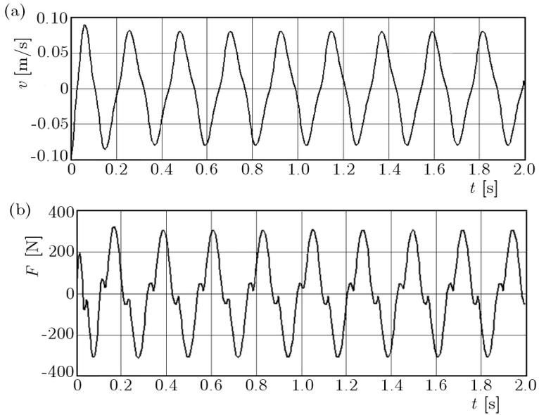
Fig. 6. Time histories of: (a) relative velocity  $v = \dot{x} - \dot{z}$ , (b) damper force  $F$
