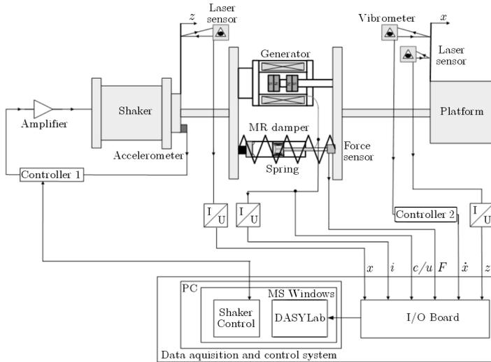
Fig. 8. Schematic diagram of the measurement and control system of the stand
