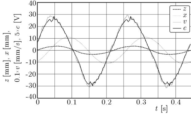
Fig. 10. Time histories of the electromotive force  $e$ , displacement of the platform  $x$  and relative velocity  $v$  under a sine excitation  $z$  with the amplitude 3.5 mm and frequency 4.5 Hz
