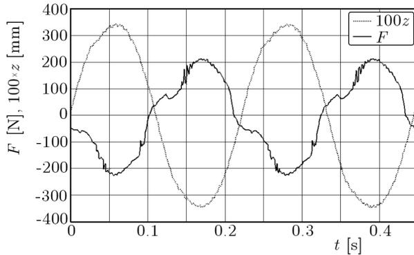
Fig. 12. Time histories of the damper force  $F$  under a sine excitation  $z$  with the amplitude 3.5 mm and frequency 4.5 Hz
