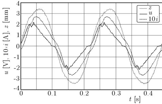
Fig. 11. Time histories of the voltage  $u$  and current  $i$  in the generator-MR damper electric circuit under a sine excitation  $z$  with the amplitude 3.5 mm and frequency 4.5 Hz
