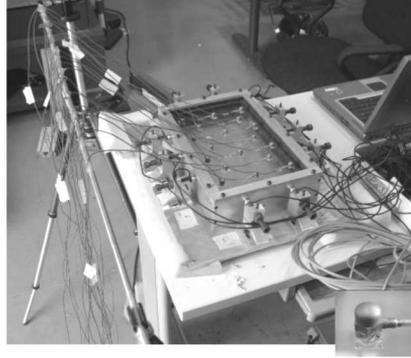
Fig. 12. Experimental modal tests on the window prototype
