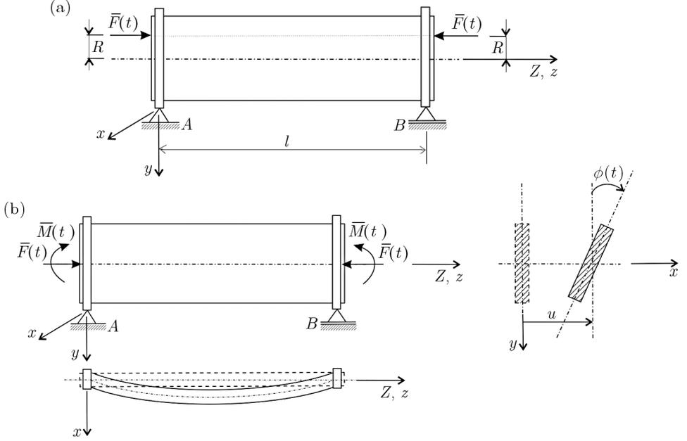
Fig. 1. Geometry of the thin-walled beam system
