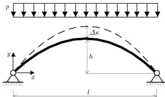
Fig. 1. Two-hinged arches (solid line: thrust line arch, dashed line: modified configuration)
