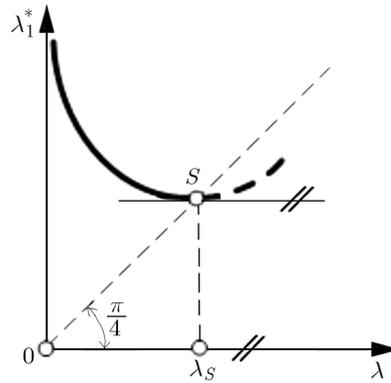
Fig. 4.  $\lambda_1^* - \lambda$  diagram for the buckling from a pure bending stress state (lateral torsional buckling)
