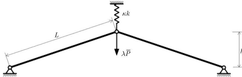
Fig. 2. *Von Mises* truss with an elastic vertical spring attached to the load point)
