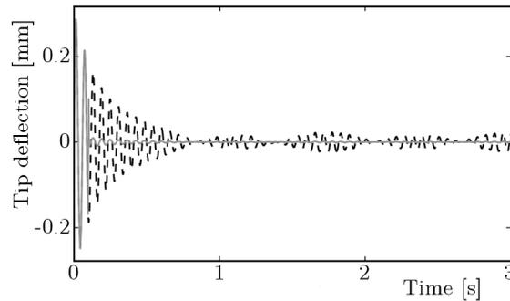
Fig. 6. Time response of vibration in the presence of a sinusoidal disturbance applying the designed robust adaptive controller (—), and without control (— —)
