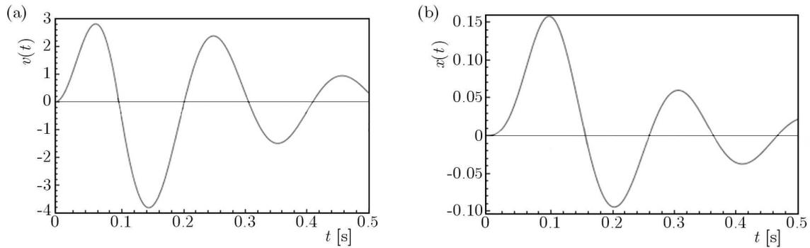
Fig. 6. Responses to the pulse loads for model 1b, (a) velocity  $v = v(t)$ , (b) displacement  $x = x(t)$
