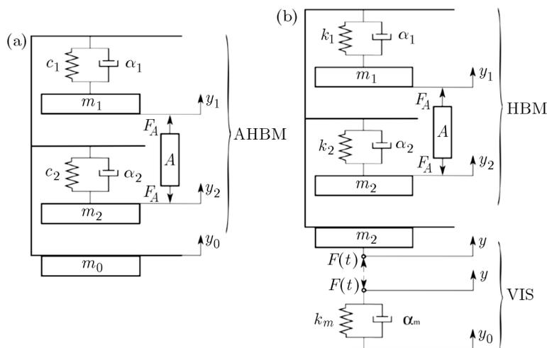
Fig. 1. Active human body model with rigid seat (a) and with passive (VIS) seat (b), Książek (1999b)
