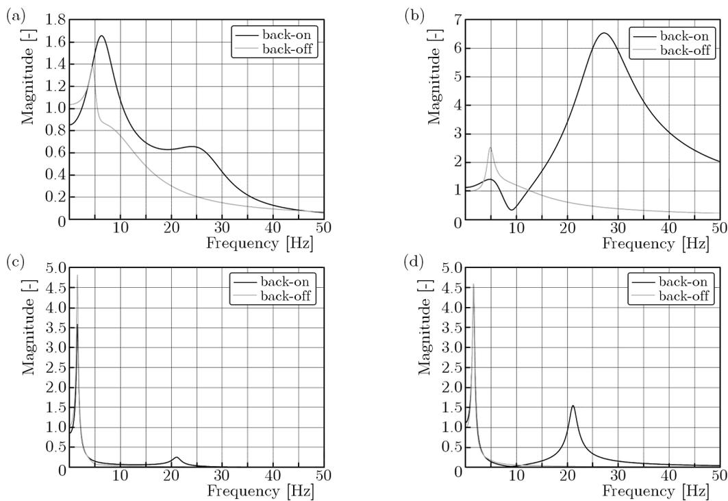
Fig. 4. Bode plot for both “back-on” and “back-off” positions in the range 0.1-50 Hz: (a) upper mass, rigid seat; (b) lower mass, rigid seat; (c) upper mass, passive seat ( $\alpha = 260$  Ns/m); (d) lower mass, passive seat ( $\alpha = 260$  Ns/m)
