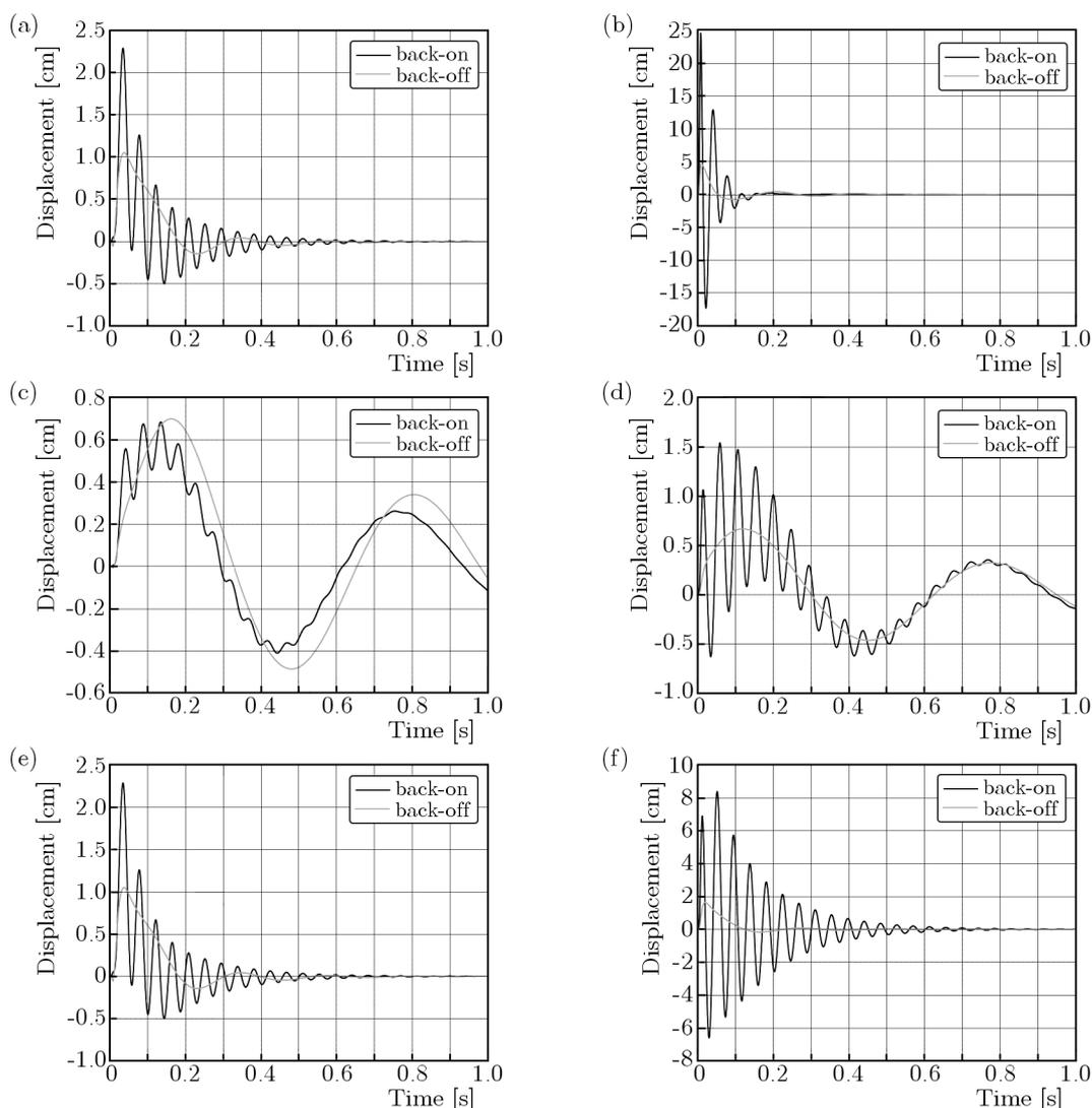
Fig. 3. Response of the human body-seat model to the impulse excitation for both “back-on” and “back-off” positions: (a) upper mass, rigid seat; (b) lower mass, rigid seat; (c) upper mass, passive seat ( $\alpha = 260$  Ns/m); (d) lower mass, passive seat ( $\alpha = 260$  Ns/m); (e) upper mass, passive seat ( $\alpha = 2600$  Ns/m); (f) lower mass, passive seat ( $\alpha = 2600$  Ns/m)
