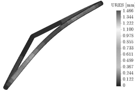
Fig. 12. Scheme of the FEM model of the triangular frame
