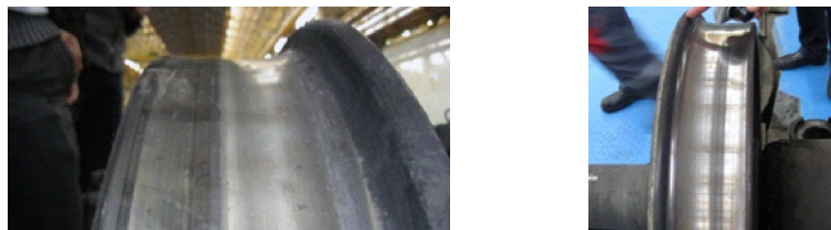
Fig. 1. Tread defects after 10 000 km passage
