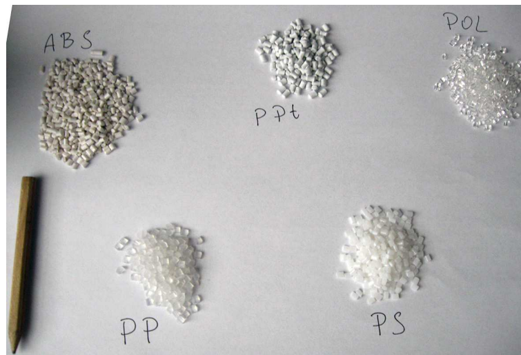
Fig. 2. Particles used in the specimen construction
