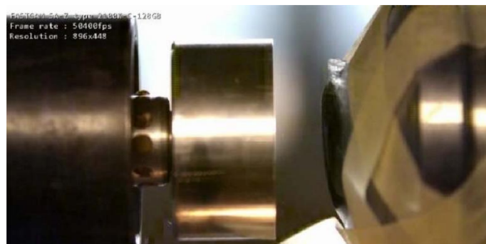
Fig. 1. Image with the projectile before impact on the cell attached to the curved surface
