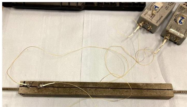
Fig. 2. Set-up of the pencil lead break test
