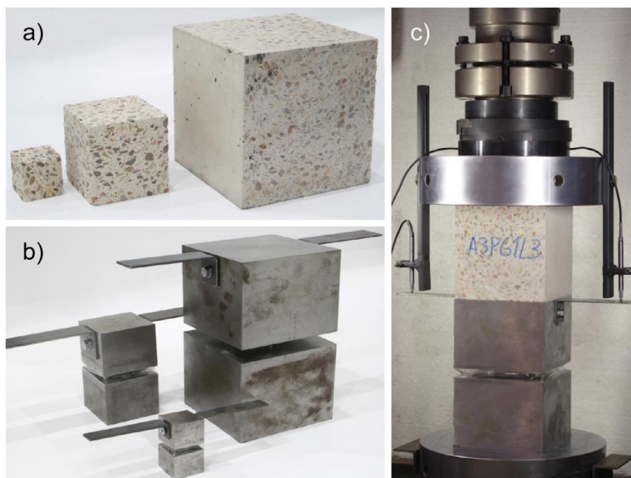
Fig. 1. (a) Cubes and (b) ball-and-socket joints of the three sizes; (c) large cube being tested
