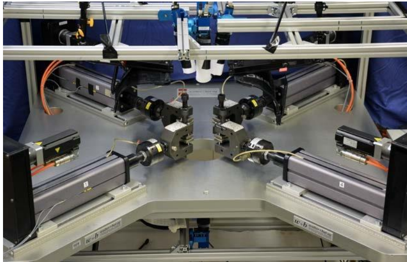
Fig. 2. Experimental Setup: Biaxial machine, digital image correlation system and lightning system
