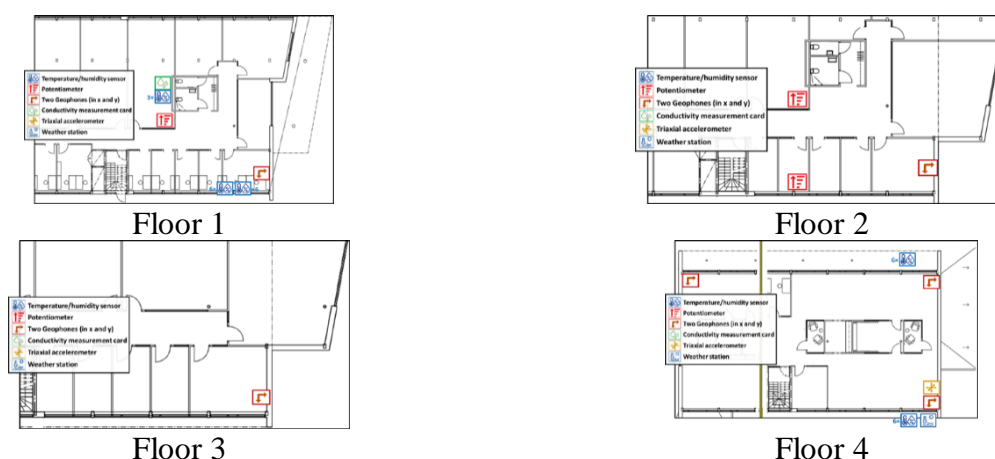
Fig. 1. Layout of the sensors and sensor groups (floor 1 to floor 4)
