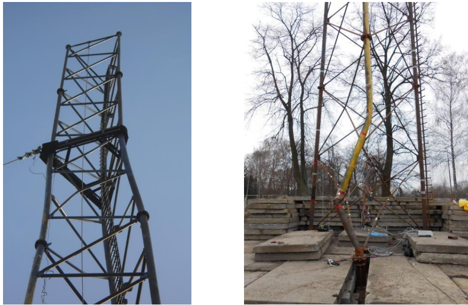
Fig. 1. Mode of failure of tower no. 1 (left) and tower no. 2 (right)
