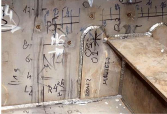
Fig. 3. Ship section tested with MagStress5D
