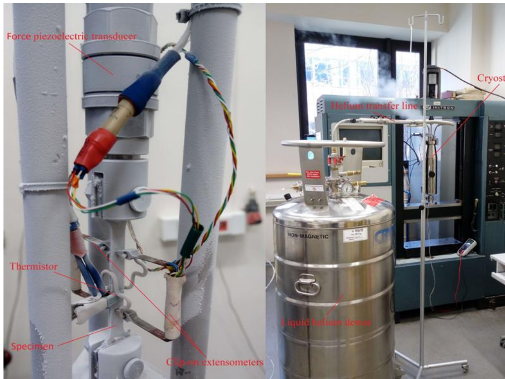
Fig 1. Experimental set-up for fracture tests at extremely low temperatures
