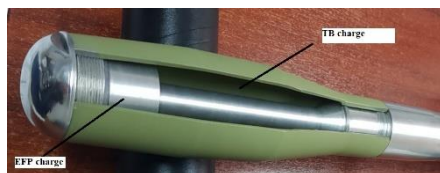
Fig. 2. EFP/TB Tandem charge test configuration
