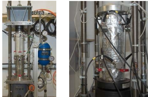
Fig. 1. Test setup for the creep and shrinkage tests: Creep test bench with one sealed and one unsealed specimen (left) and detail view of a sealed specimen (right), showing displacement transducers and piezoelectric transducers for acoustic emission measurements
