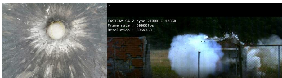
Figure 4. The effect on 10 mm target steel plate and on the concrete test building.
