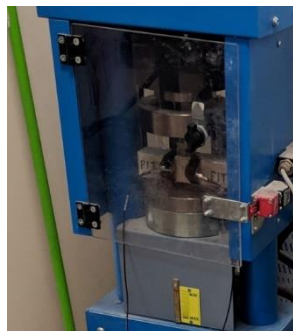
Fig. 1. Positioning of the R15 sensors during three-point bending
