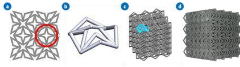
Fig. 2. The general view of lattice design process (a) 2D structure, (b) an exemplary unit cell (c) 3D lattice structure (d) fabricated via SLS technique specimen
